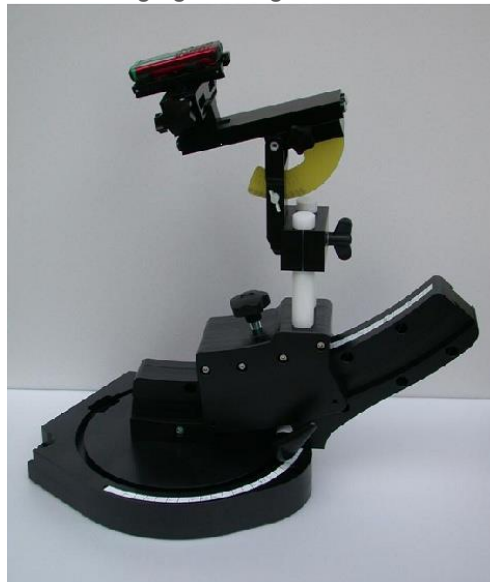
Device holder supplied by SPEAG
