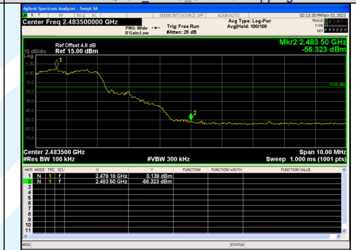
Out Of Band Emission(Right) 8DPSK_3-DH5_Channel Hopping
