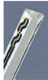
Figure E.2.2 Probe Thick-Film Technique
