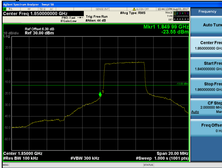
LTE Band 2 / 10MHz / QPSK - RB Size/Offset (25/0)
