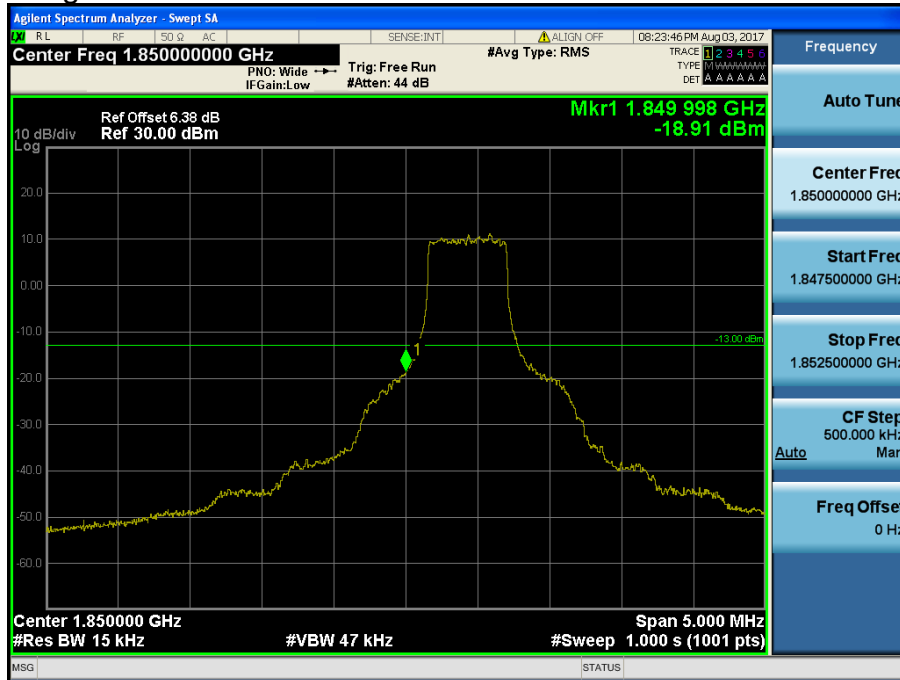
LTE Band 2 / 1.4MHz / QPSK - RB Size/Offset (3/0)
