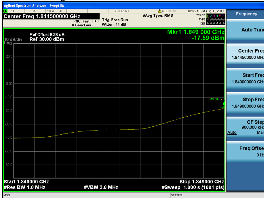
LTE Band 2 / 10MHz / QPSK - RB Size/Offset (25/0)
