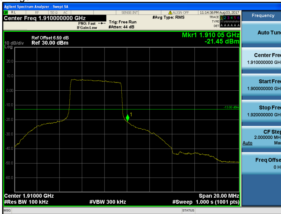
LTE Band 2 / 10MHz / QPSK - RB Size/Offset (25/25)
