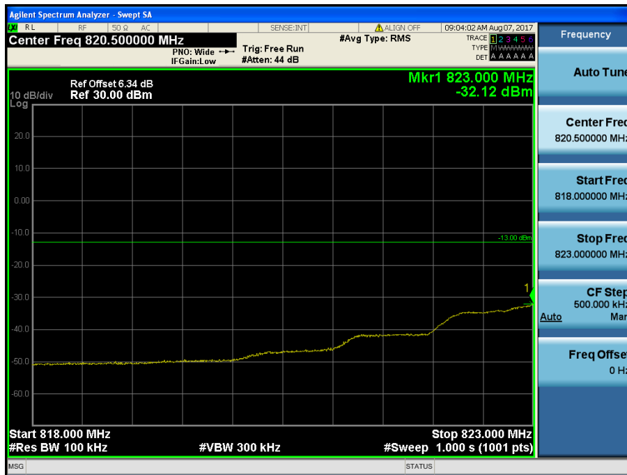
LTE Band 5 / 1.4MHz / QPSK - RB Size/Offset (6/0)
