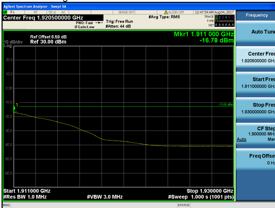
LTE Band 2 / 20MHz / QPSK - RB Size/Offset (50/50)
