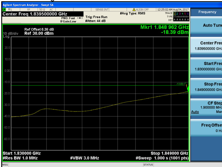
LTE Band 2 / 20MHz / QPSK - RB Size/Offset (100/0)
