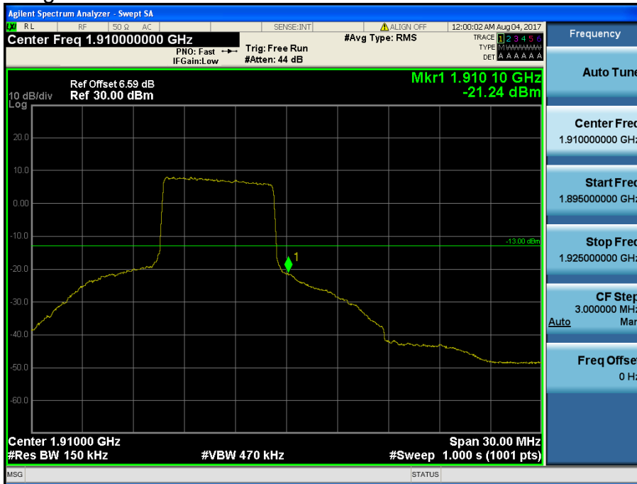
LTE Band 2 / 15MHz / QPSK - RB Size/Offset (36/39)
