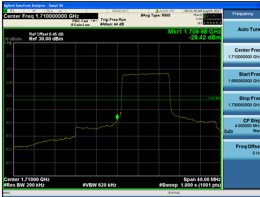
LTE Band 4 / 20MHz / QPSK - RB Size/Offset (50/0)
