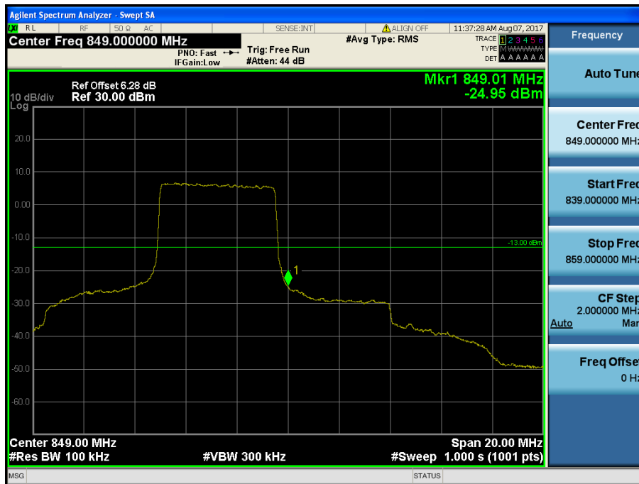
LTE Band 5 / 10MHz / QPSK - RB Size/Offset (25/25)
