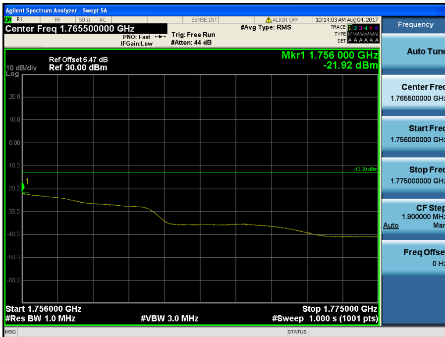
LTE Band 4 / 20MHz / QPSK - RB Size/Offset (50/50)
