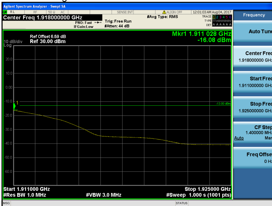
LTE Band 2 / 15MHz / QPSK - RB Size/Offset (36/39)
