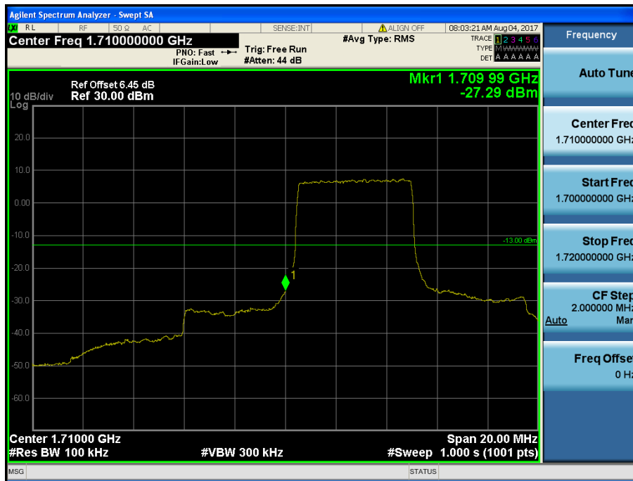
LTE Band 4 / 10MHz / QPSK - RB Size/Offset (25/0)
