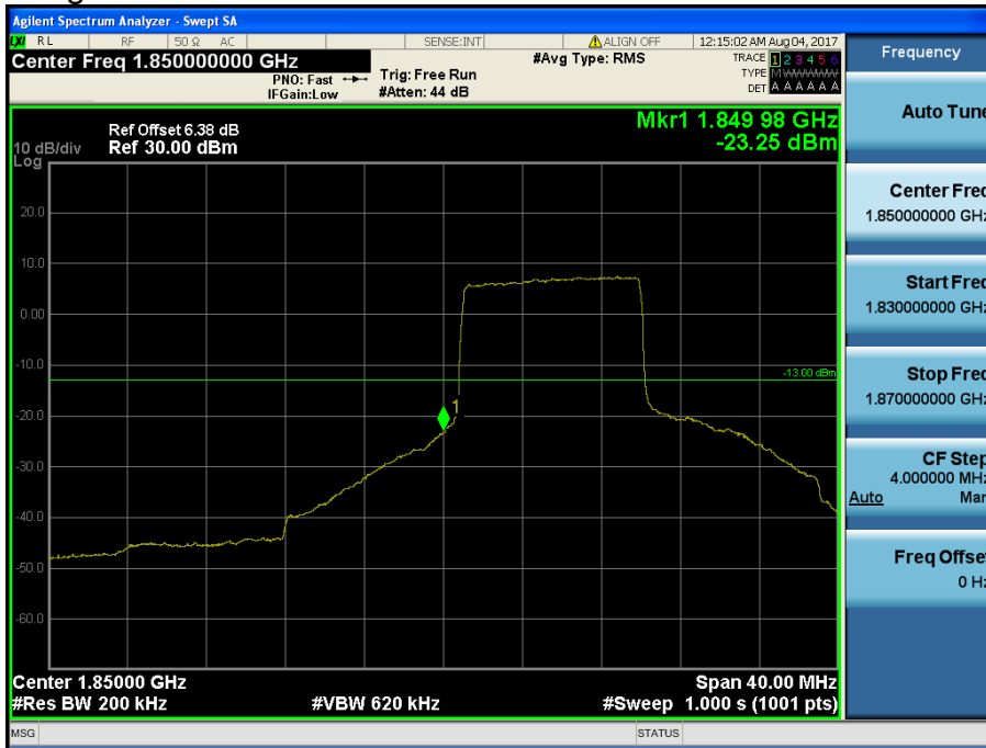
LTE Band 2 / 20MHz / QPSK - RB Size/Offset (50/0)
