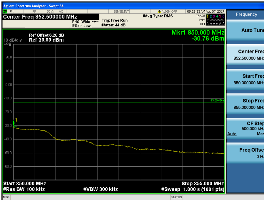
LTE Band 5 / 1.4MHz / QPSK - RB Size/Offset (6/0)
