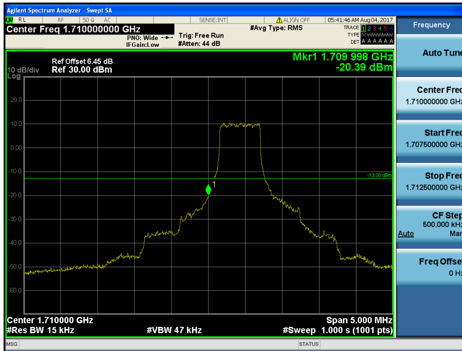
LTE Band 4 / 1.4MHz / QPSK - RB Size/Offset (3/0)
