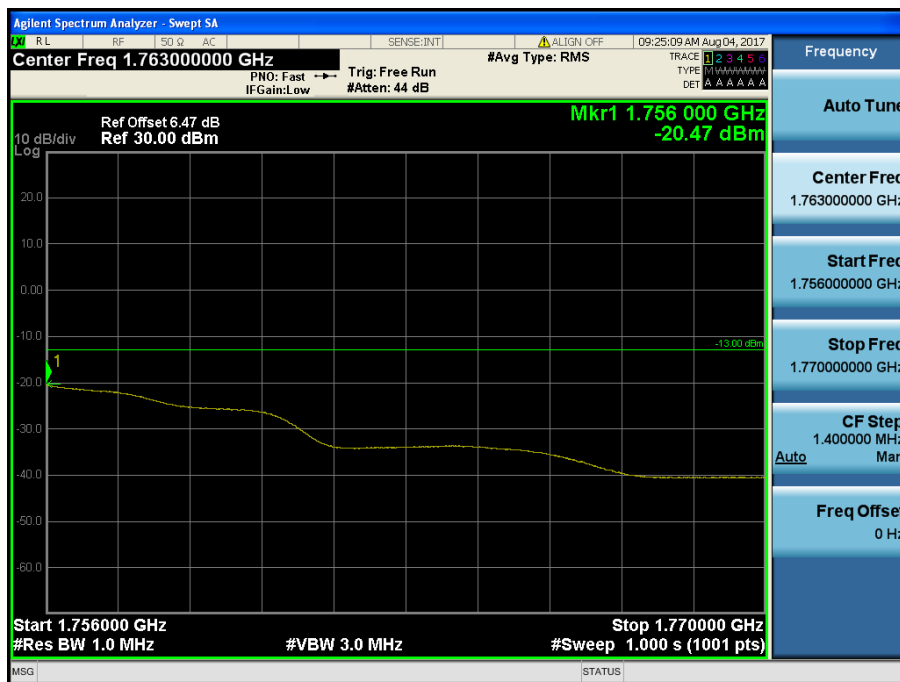
LTE Band 4 / 15MHz / QPSK - RB Size/Offset (36/39)
