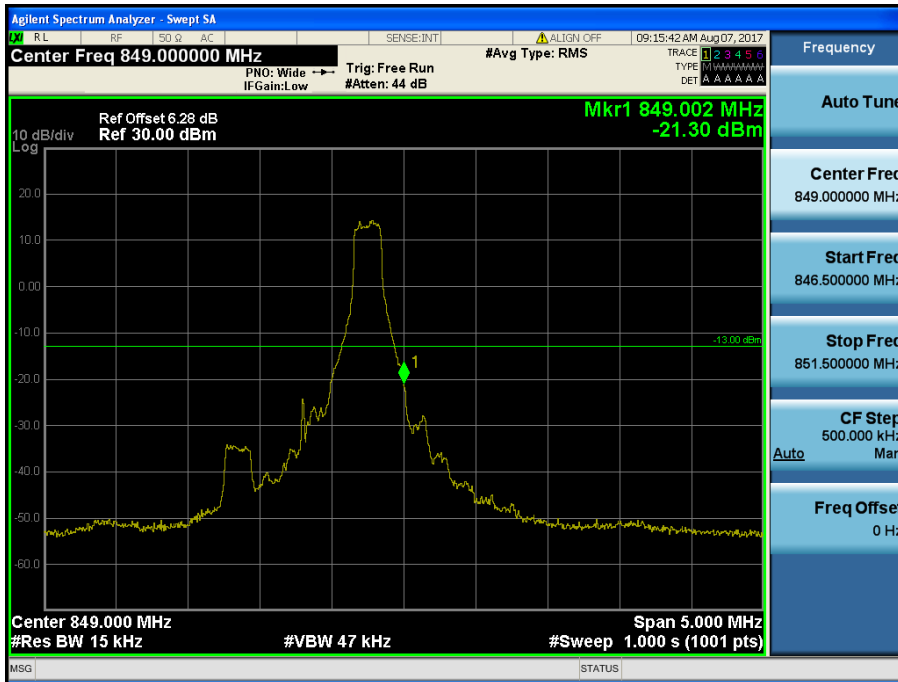
LTE Band 5 / 1.4MHz / QPSK - RB Size/Offset (1/5)
