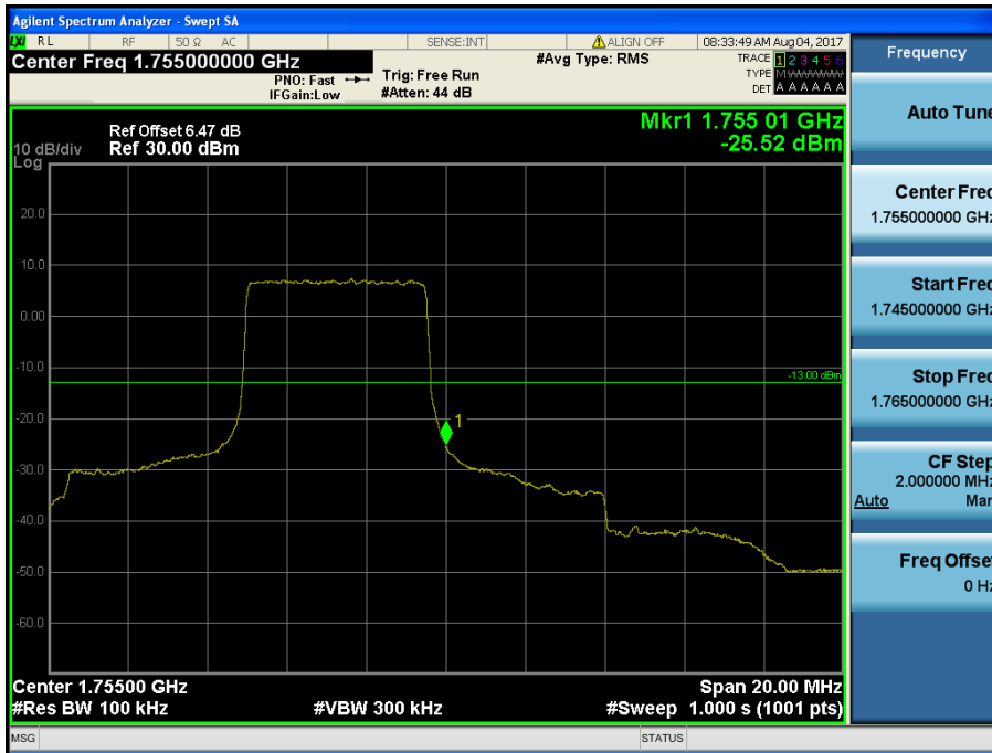
LTE Band 4 / 10MHz / QPSK - RB Size/Offset (25/25)
