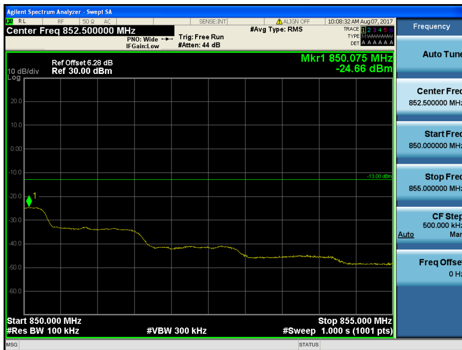
LTE Band 5 / 3MHz / QPSK - RB Size/Offset (8/7)
