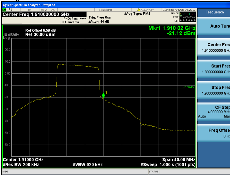
LTE Band 2 / 20MHz / QPSK - RB Size/Offset (50/50)
