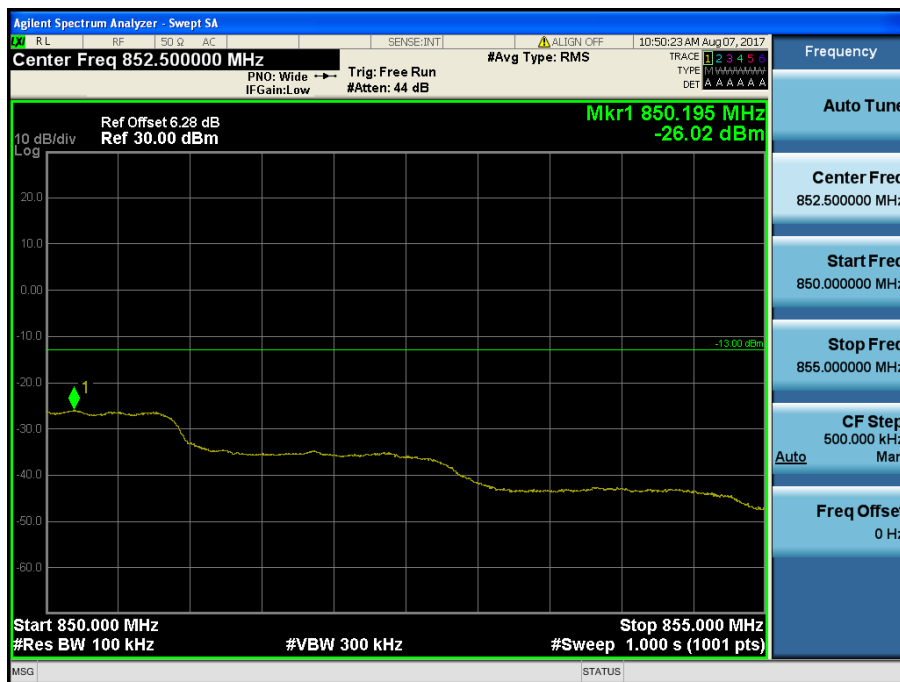
LTE Band 5 / 5MHz / QPSK - RB Size/Offset (12/13)
