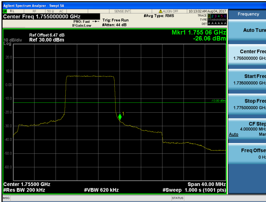
LTE Band 4 / 20MHz / QPSK - RB Size/Offset (50/50)
