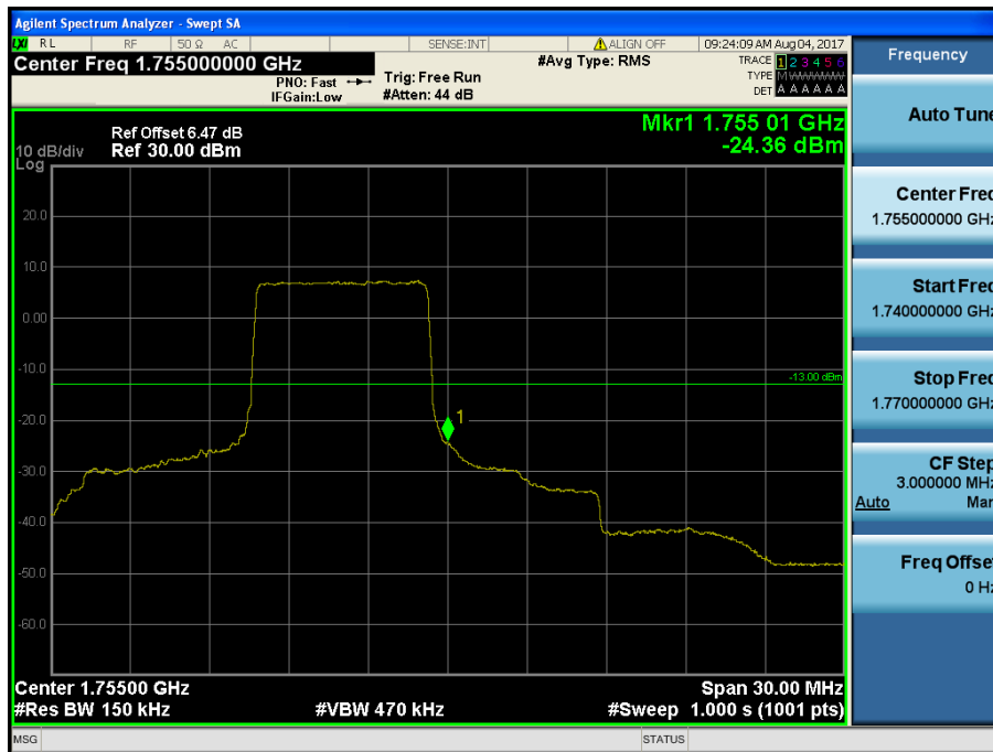
LTE Band 4 / 15MHz / QPSK - RB Size/Offset (36/39)
