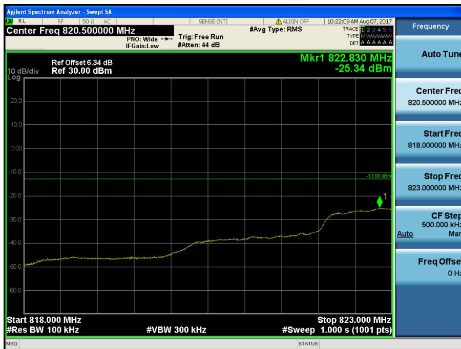
LTE Band 5 / 5MHz / QPSK Offset/Size (12/0)
