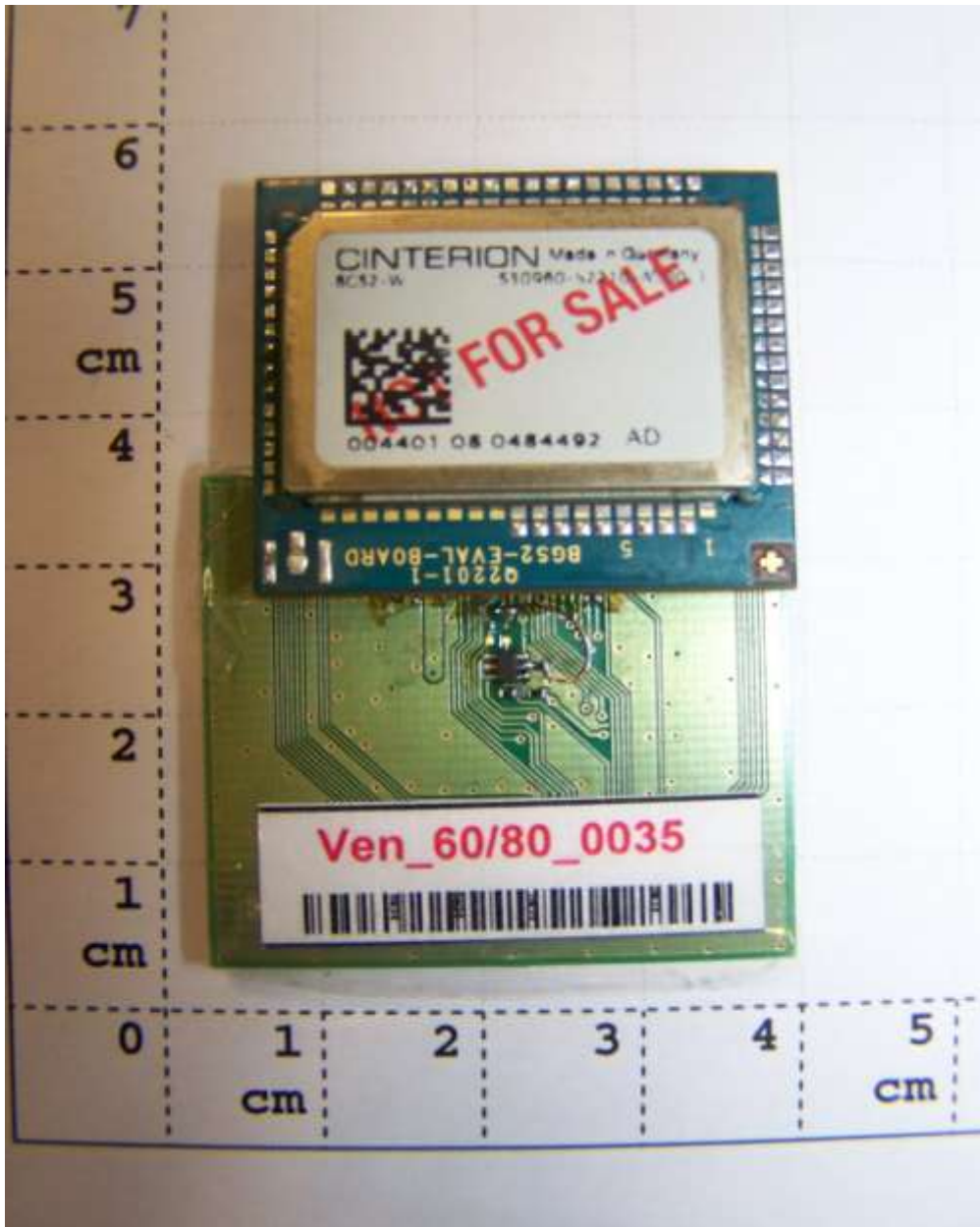
Photograph 4: EUT F+ Adapter board for BGS2-W bottom side
