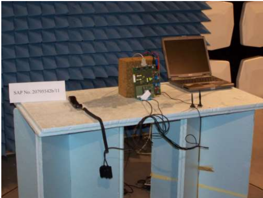
Photograph 1: Radiated measurement set-up at SAR (Semi-Anechoic-Room)
