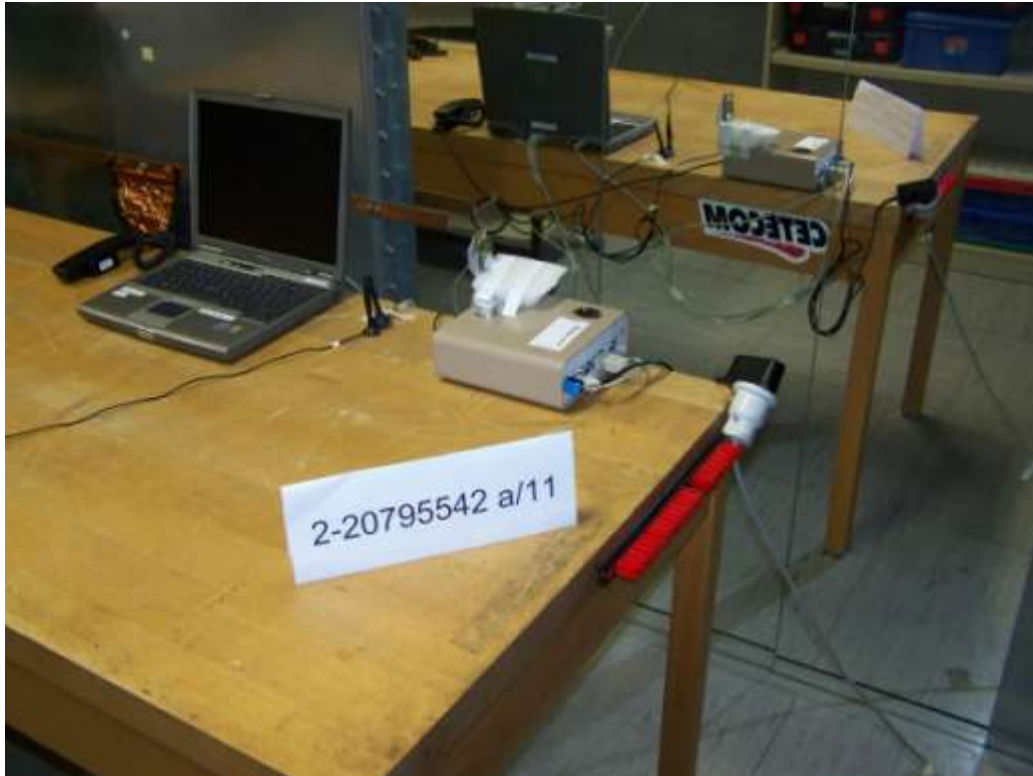
Photograph 3: Conducted emissions on AC line measurements
