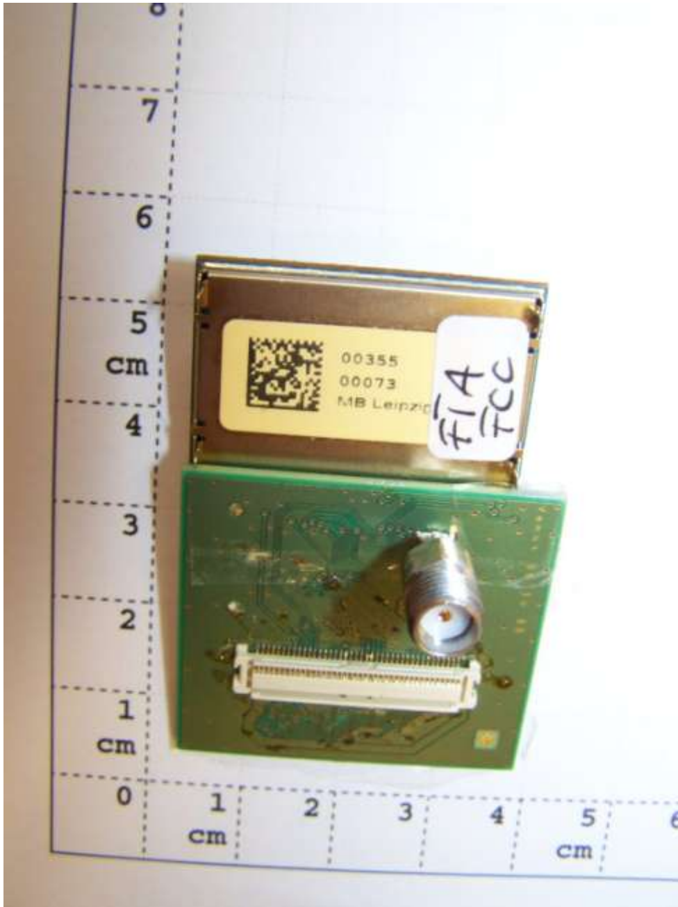
Photograph 3: EUT F – top side PCB with Hirose SMA adapter
