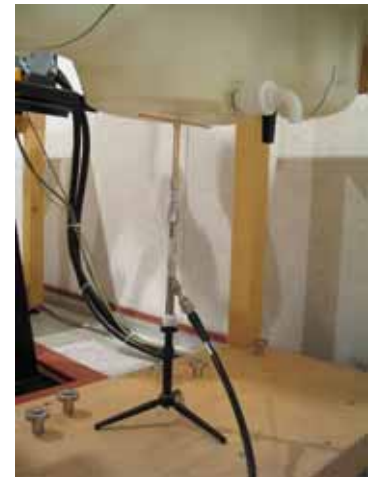
Photo of the dipole Antenna
