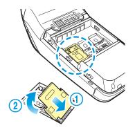
① Push the USIM card holder to 'OPEN' direction then lift up.
