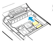
Push the top of the USIM card to slide it out in the arrow direction.
