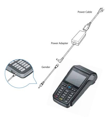
As you see in the picture, connect the adapter with the power cable to charge the power.
