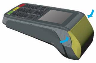
Remove any partial roll of paper in the printer tray by lifting up.
