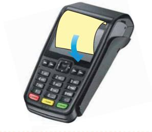
The printer cover can open if the Receipt is pulled backward.
