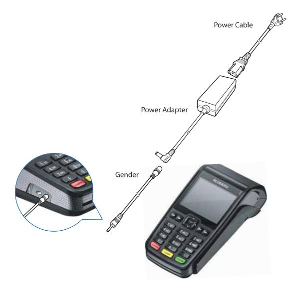
As you see in the picture, connect the adapter with the power cable to charge the power.
