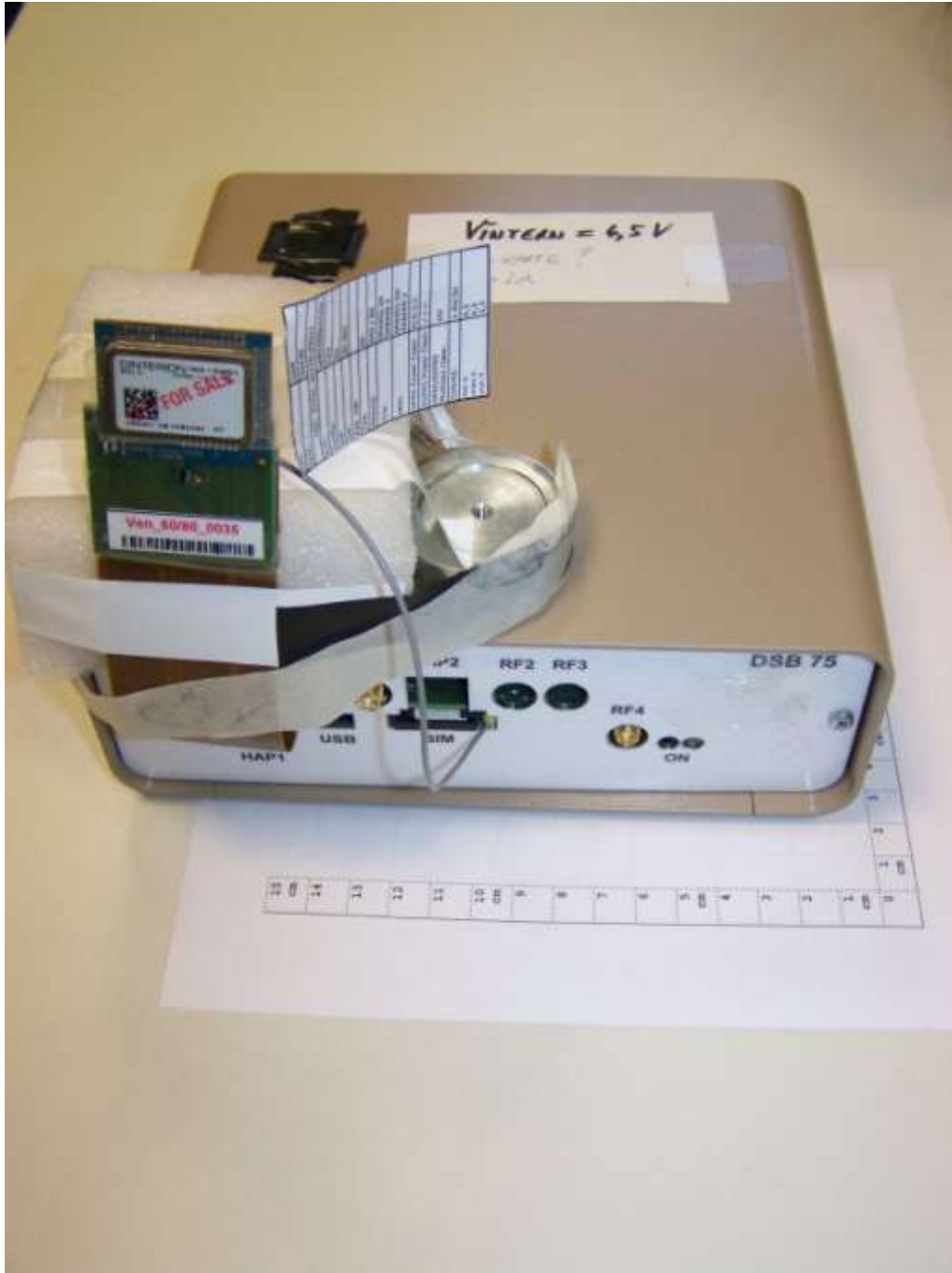
Photograph 5: Modules connection (flexible flat ribbon and adapter) to DSB75 Box (EUT D + E)
