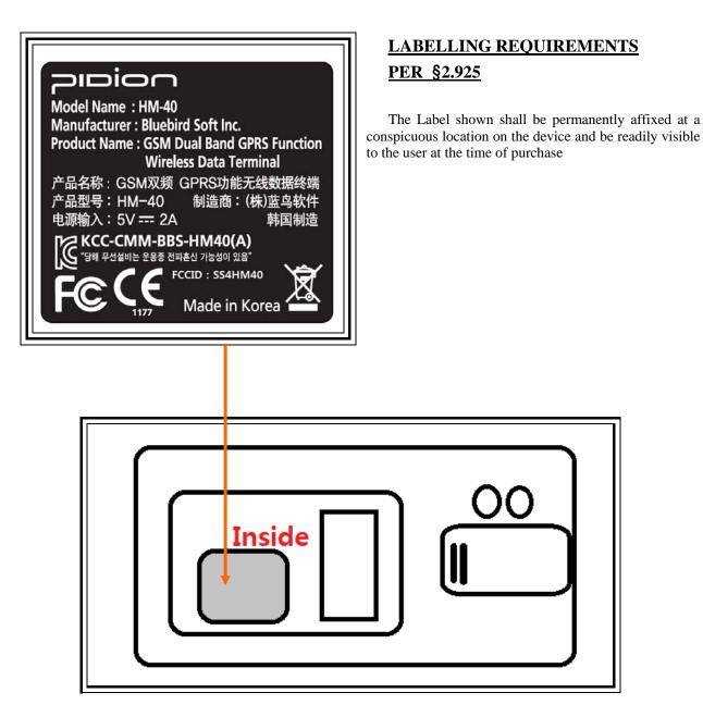
The label is attached to this device by an adhesive. The adhesive is permanent type with strong strength. Additionally, the label is readily to the purchaser at the time of purchase.
