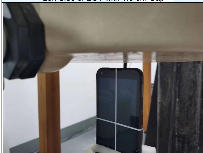
Top Side of EUT with 1.0 cm Gap
