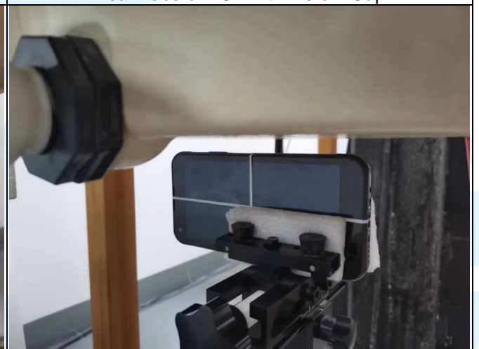
Right Side of EUT with 1.0 cm Gap
