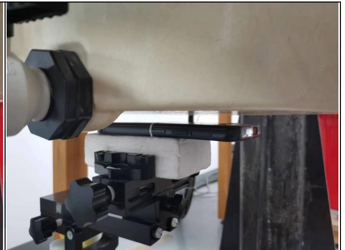
Rear Face of EUT with 1.0 cm Gap
