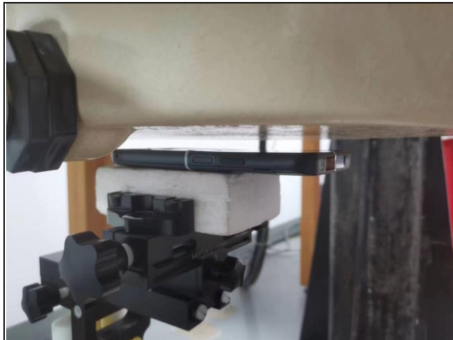
Front Face of EUT with 1.0 cm Gap
