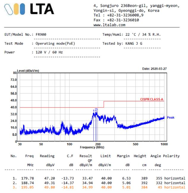
Remarks: C.F (Correction Factor) = Antenna factor + Cable loss - Preamp gain
