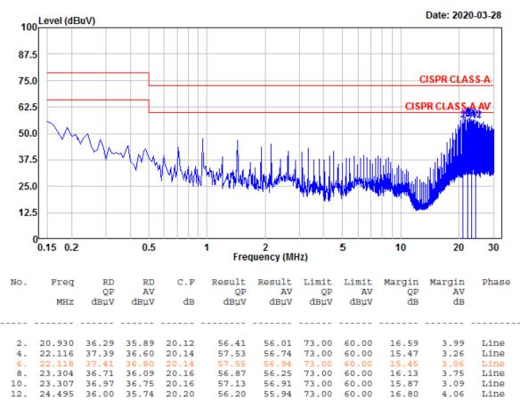
Remarks: C.F (Correction Factor) = Insertion loss + Cable loss + Pulse Limiter
