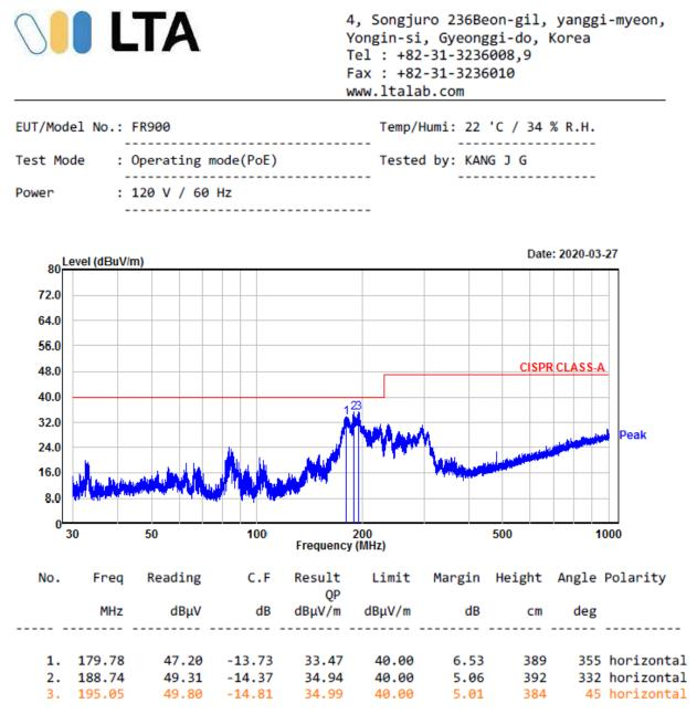
Remarks: C.F (Correction Factor) = Antenna factor + Cable loss - Preamp gain
