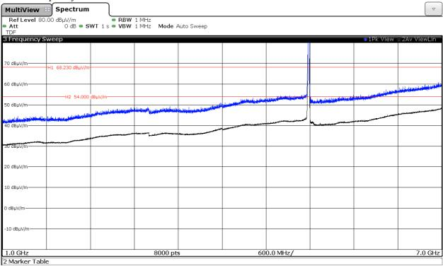
Note: The peak above the limit is the carrier frequency. This plot is valid for both Chain A and Chain B.
