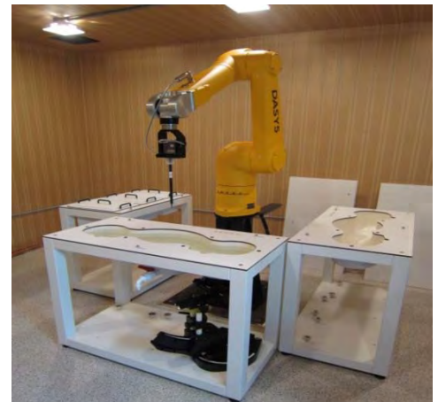
Figure E.7.1 DASY5 Test System
