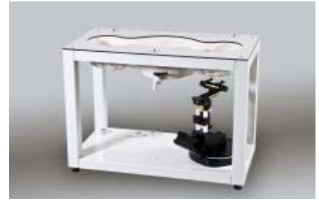
Figure E.5.1 SAM Twin Phantom
