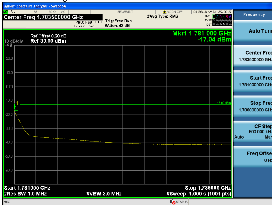
LTE Band 66 / 1.4MHz / QPSK - RB Size/Offset (1/2)
