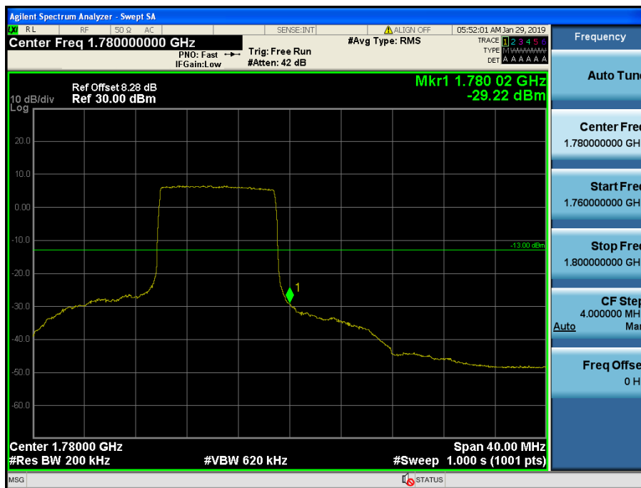
LTE Band 66 / 20MHz / QPSK - RB Size/Offset (50/50)
