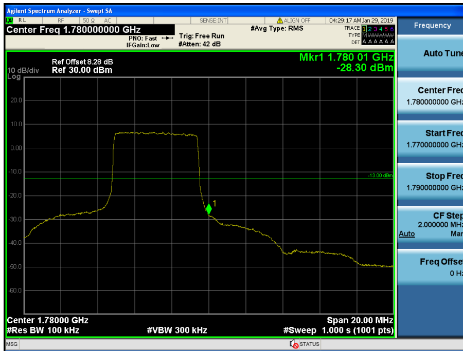
LTE Band 66 / 10MHz / QPSK - RB Size/Offset (25/25)
