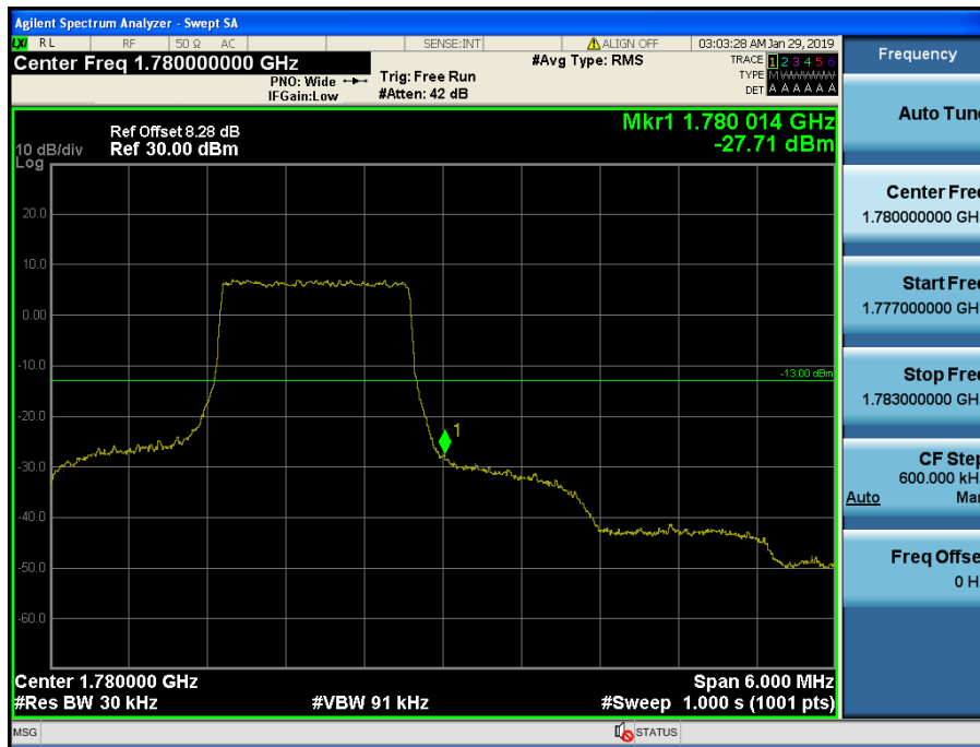
LTE Band 66 / 3MHz / QPSK - RB Size/Offset (8/7)
