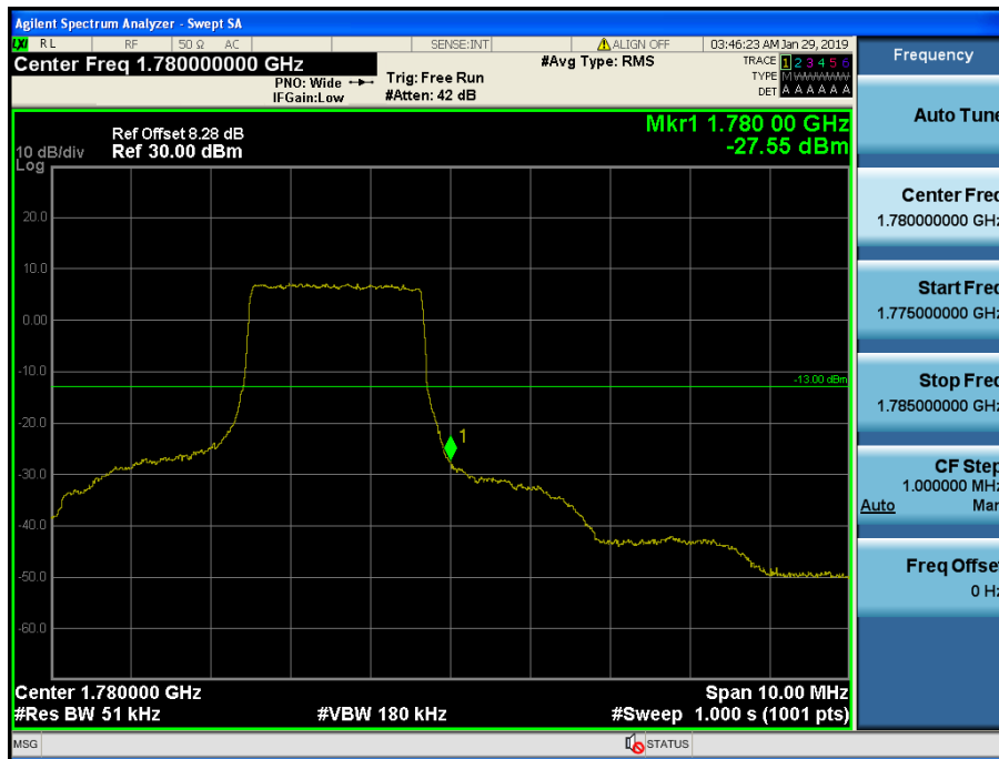
LTE Band 66 / 5MHz / QPSK - RB Size/Offset (12/13)
