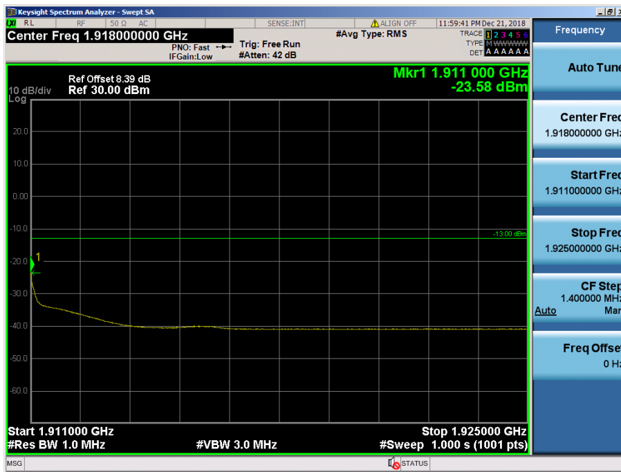
LTE Band 2 / 15MHz / QPSK - RB Size/Offset (1/74)
