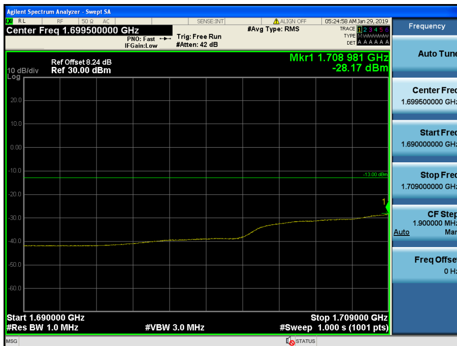
LTE Band 66 / 20MHz / QPSK - RB Size/Offset (50/0)
