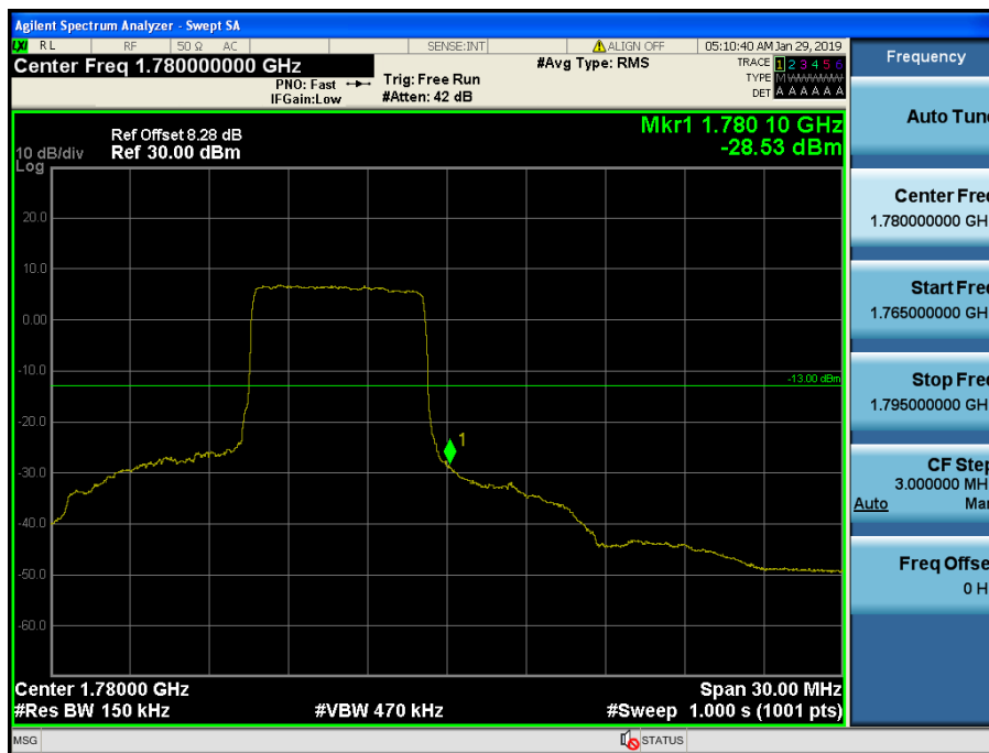
LTE Band 66 / 15MHz / QPSK - RB Size/Offset (36/39)
