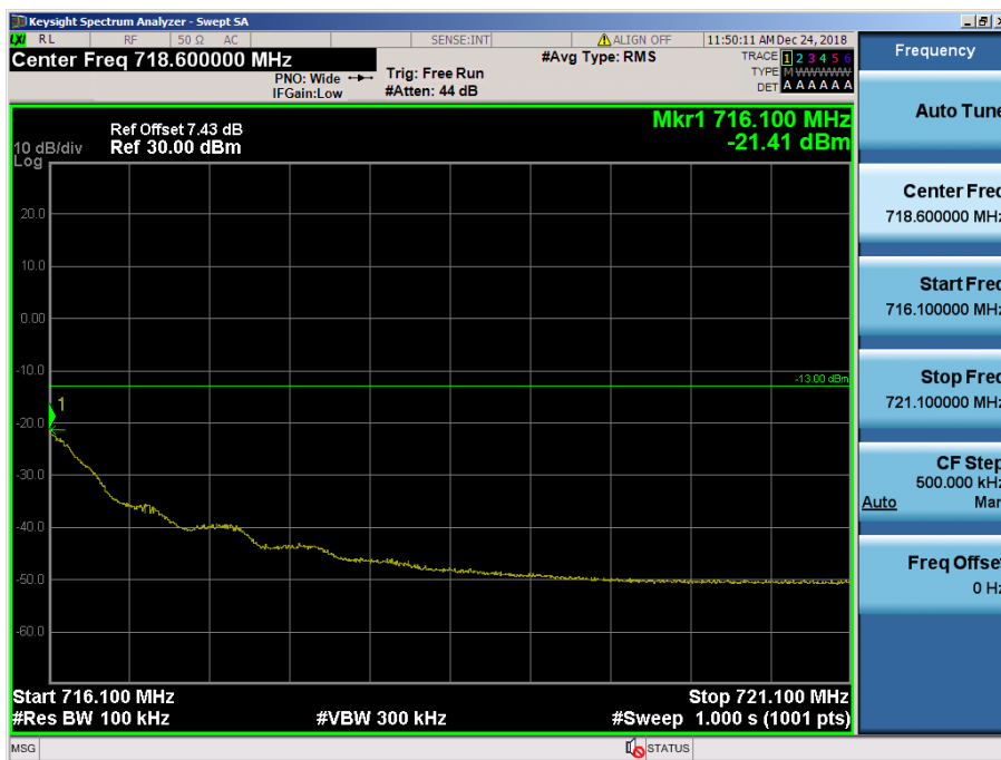
LTE Band 12 / 1.4MHz / QPSK - RB Size/Offset (3/3)
