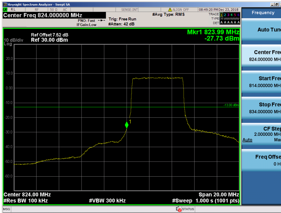
LTE Band 5 / 10MHz / QPSK - RB Size/Offset (25/0)
