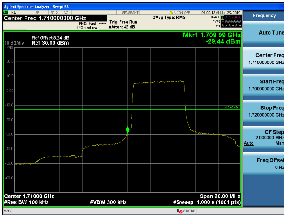
LTE Band 66 / 10MHz / QPSK - RB Size/Offset (25/0)
