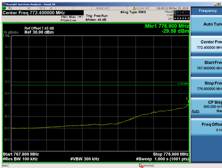
LTE Band 13 / 10MHz / QPSK - RB Size/Offset (25/0)
