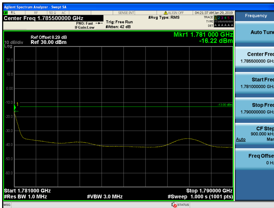
LTE Band 66 / 10MHz / QPSK - RB Size/Offset (1/49)
