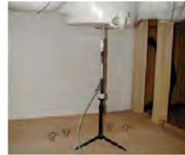
Figure 11.1 Dipole Verification Test Setup Diagram & Photo
