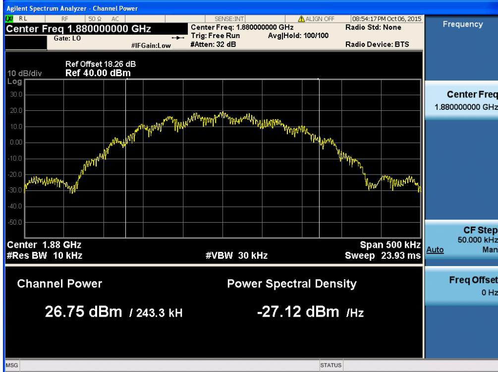
$$\text{PAR (dB)} = \text{P}_{\text{Pk}} (\text{dBm}) - \text{P}_{\text{Avg}} (\text{dBm}) = 30.94 \text{ dBm} - 26.75 \text{ dBm} = 4.19 \text{ dB}$$
