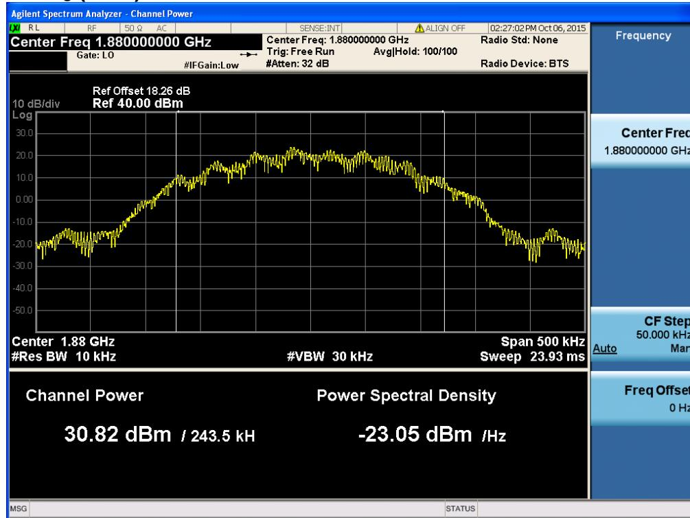
$$\text{PAPR (dB)} = P_{Pk} (\text{dBm}) - P_{Avg} (\text{dBm}) = 31.06 \text{ dBm} - 30.82 \text{ dBm} = 0.24 \text{ dB}$$
