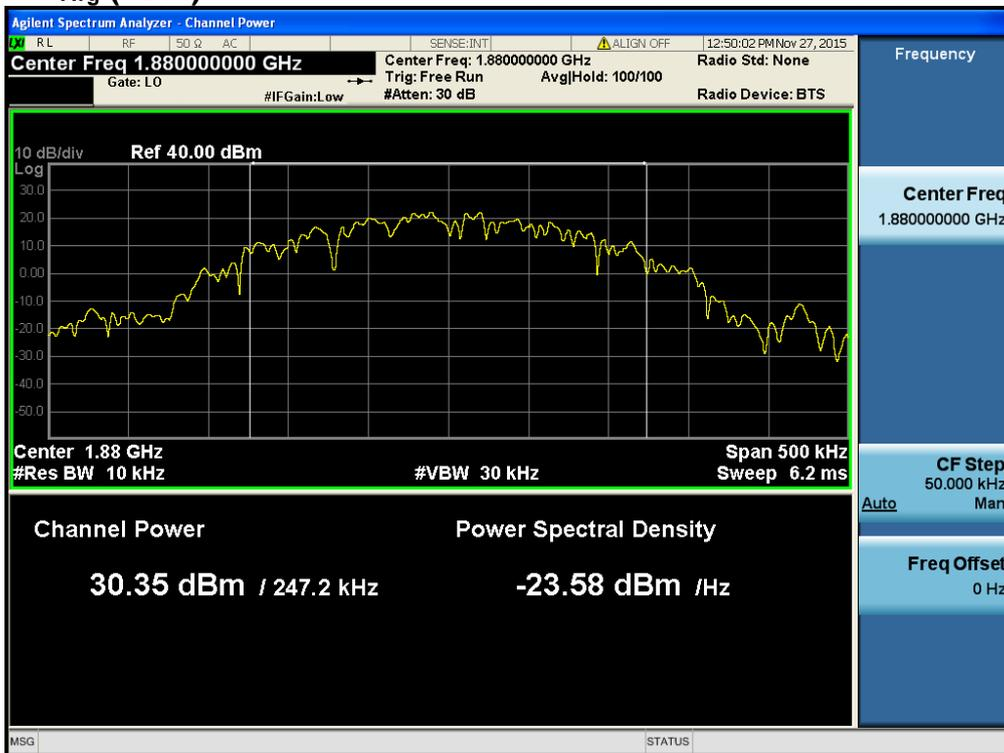
$$\text{PAPR (dB)} = P_{pk} \text{ (dBm)} - P_{avg} \text{ (dBm)} = 30.92 \text{ dBm} - 30.35 \text{ dBm} = 0.57 \text{ dB}$$
