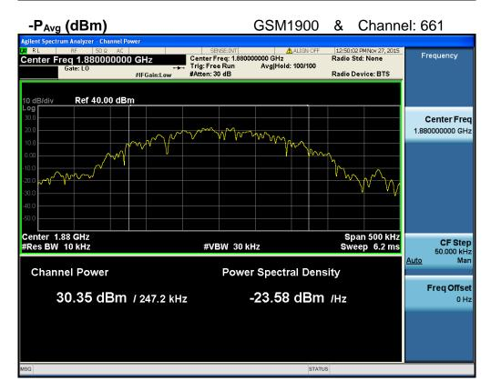
PAPR (dB) =  $P_{Pk}$  (dBm) -  $P_{Avg}$  (dBm) = 30.92 dBm - 30.35 dBm = 0.57 dB
