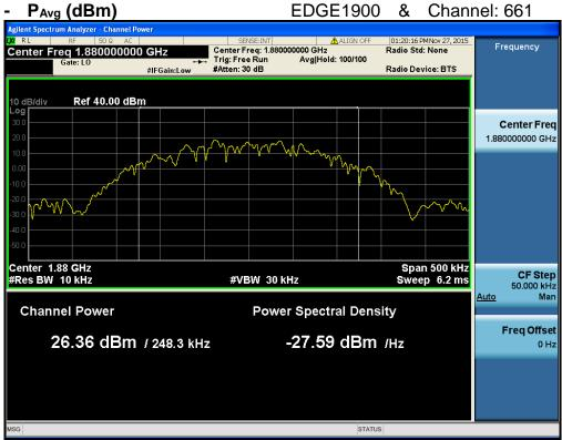
$PAR (dB) = P_{Pk} (dBm) - P_{Avg} (dBm) = 30.84 dBm - 26.36 dBm = 4.48 dB$
