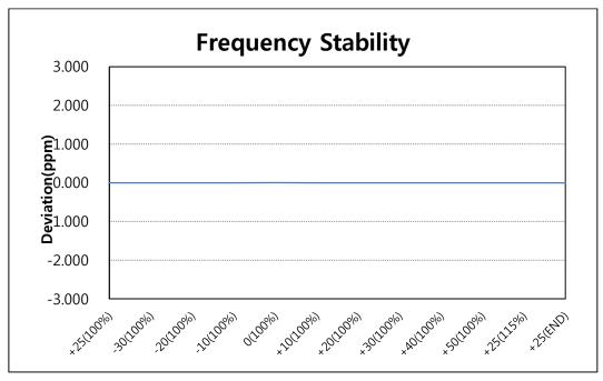
**Note.** Based on the results of the frequency stability test at the center channel the frequency deviation results measured are very small. as such it is determined that the channels at the band edge would remain inband when the maximum measured frequency deviation noted during the frequency stability tests is applied. therefore the device is determined to remain operating in band over the temperature and voltage range as tested.
