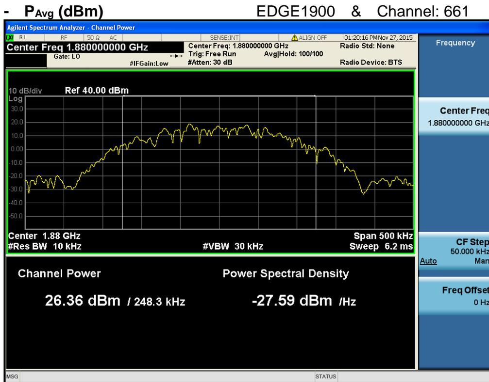
$$PAR (dB) = P_{pk} (dBm) - P_{avg} (dBm) = 30.84 \text{ dBm} - 26.36 \text{ dBm} = 4.48 \text{ dB}$$
