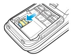
① With the USIM card and storage card compartment opened, lift the storage card holder flap to open it.
