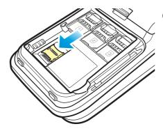
① Open the storage card holder by lifting up the flap.
