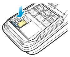
② Insert the microSD card into the storage card holder with its gold contacts facing out.
