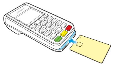
Insert IC card. IC chip needs to go in first. Please make sure that insert the card all the way in.
