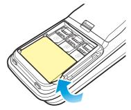
② Lift the battery in the direction of the arrow.
