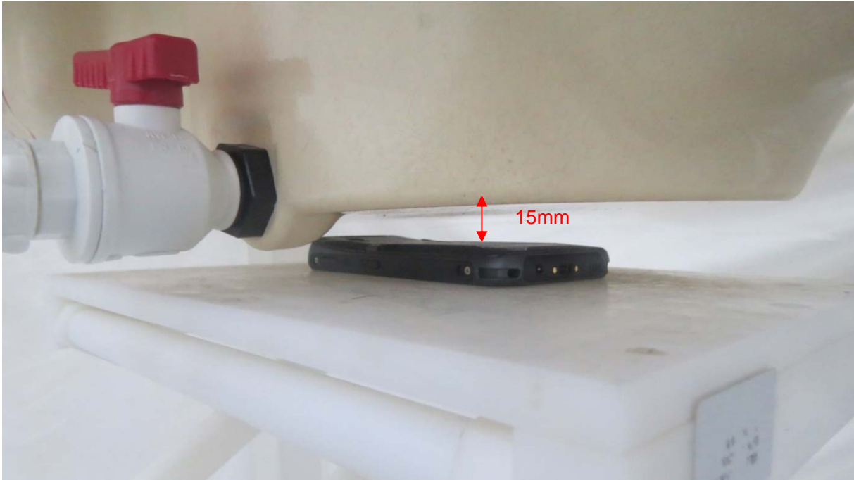
Picture 5: Back Side, the distance from handset to the bottom of the Phantom is 15mm
