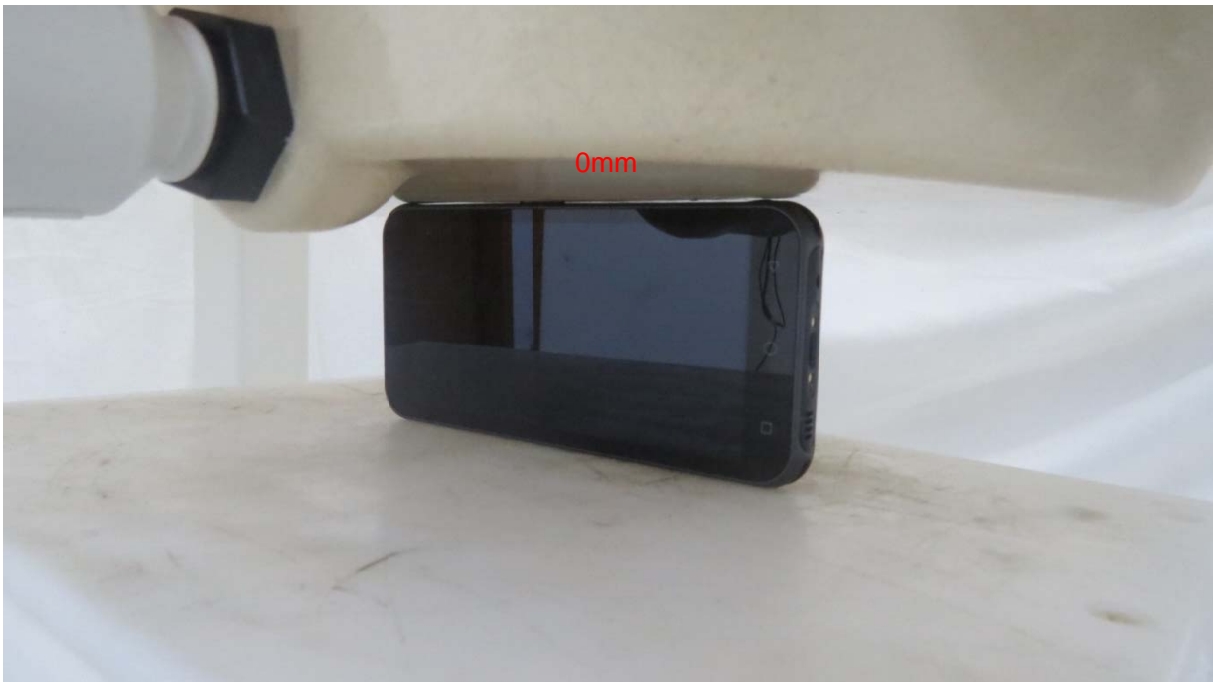
Picture 16: Right Edge, the distance from handset to the bottom of the Phantom is 0mm
