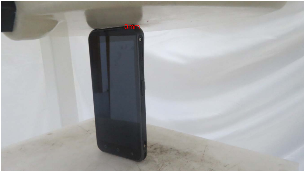
Picture 17: Top Edge, the distance from handset to the bottom of the Phantom is 0mm
