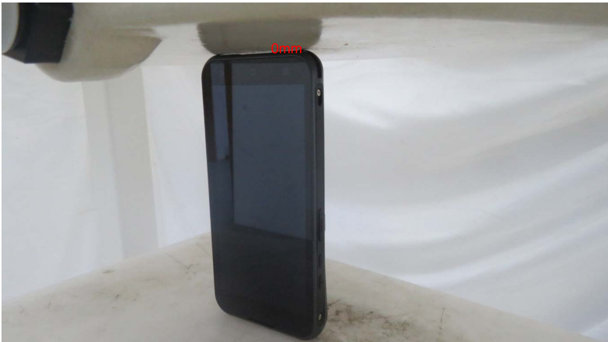
Picture 18: Bottom Edge, the distance from handset to the bottom of the Phantom is 0mm
