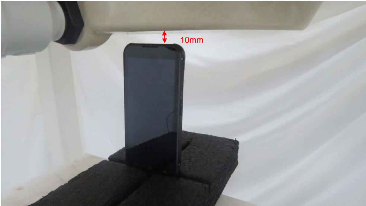
Picture 11: Top Edge, the distance from handset to the bottom of the Phantom is 10mm
