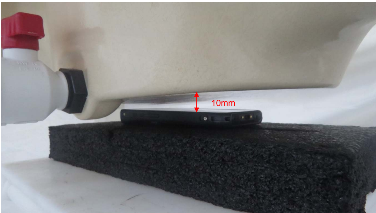
Picture 8: Front Side, the distance from handset to the bottom of the Phantom is 10mm
