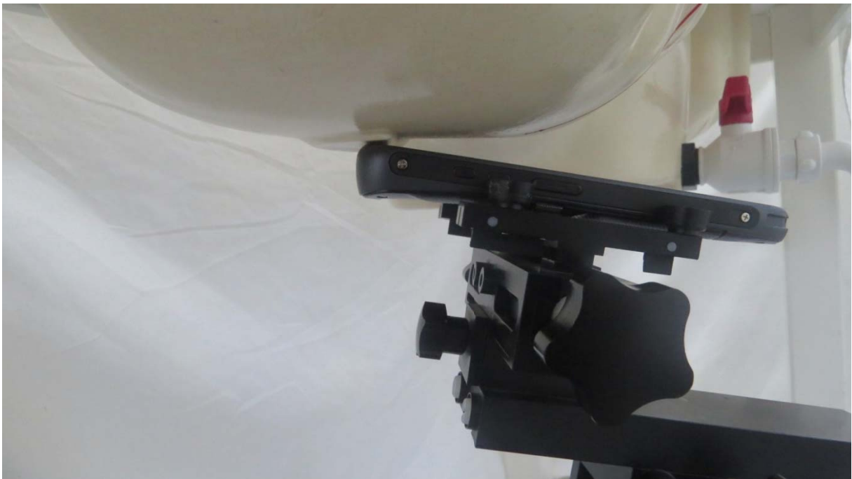
Picture 4: Right Hand Tilt 15 Degree Position
