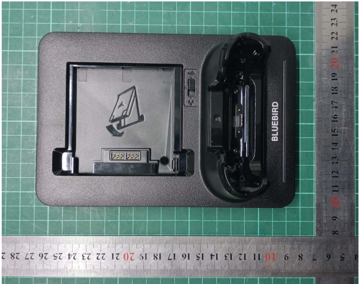
c: Charging dock
