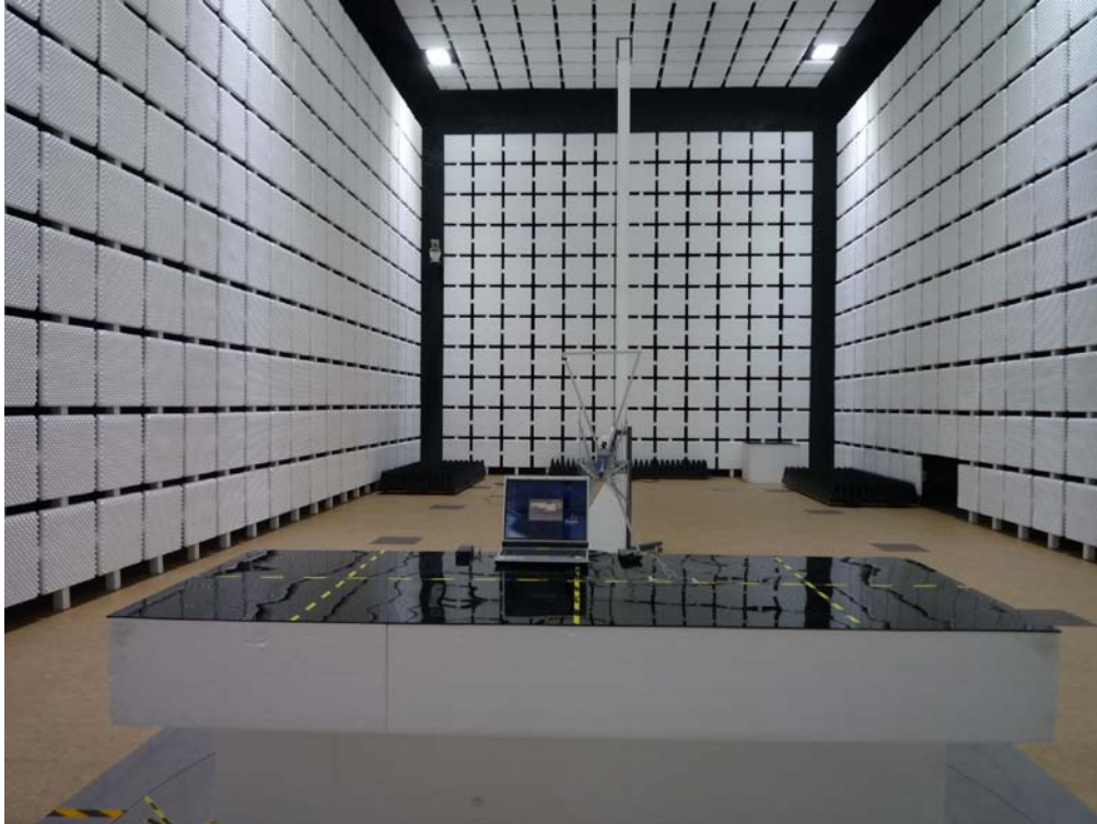
Radiated RF measurement (Above 30 MHz)
