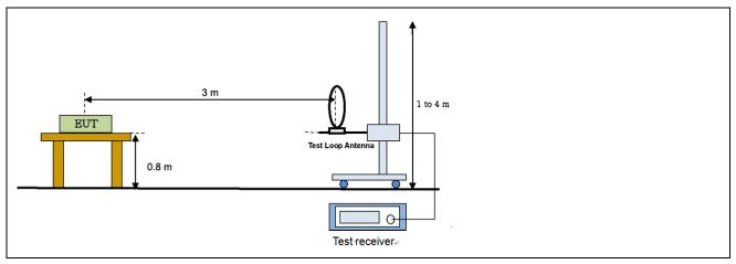
Radiated emission setup, Below 1 000 MHz
