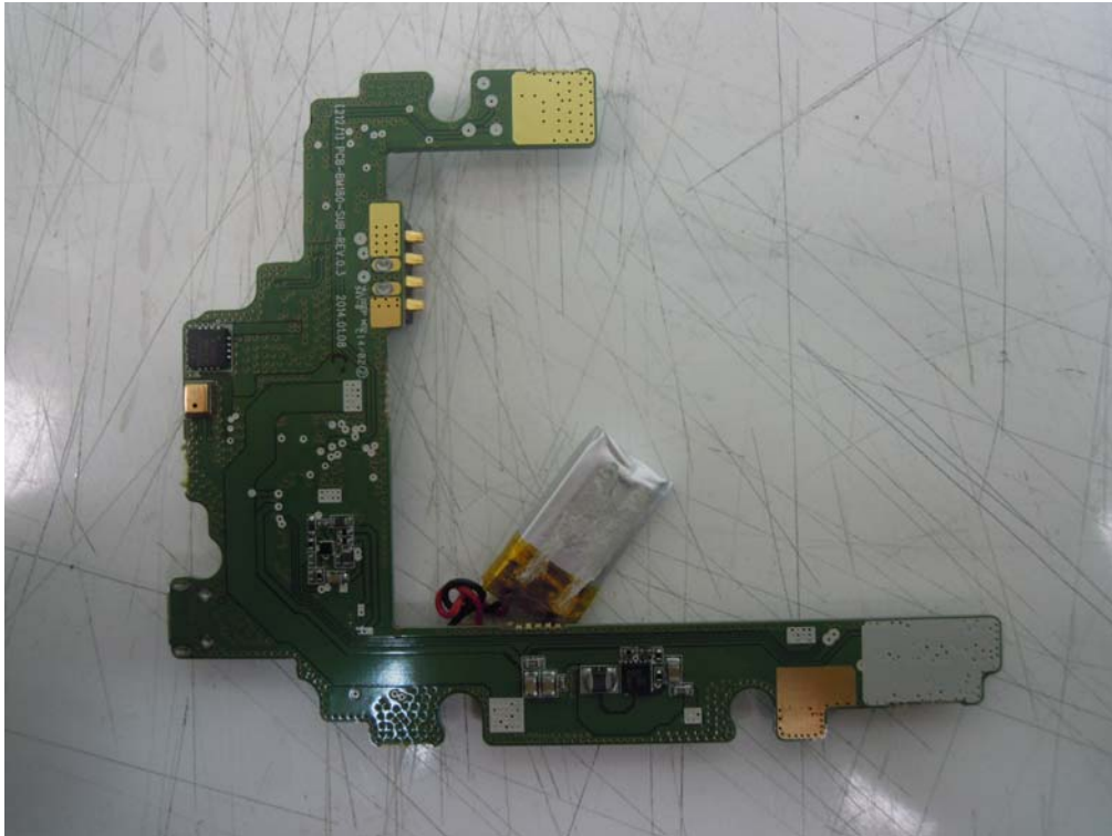
[Sub control board Rear]
