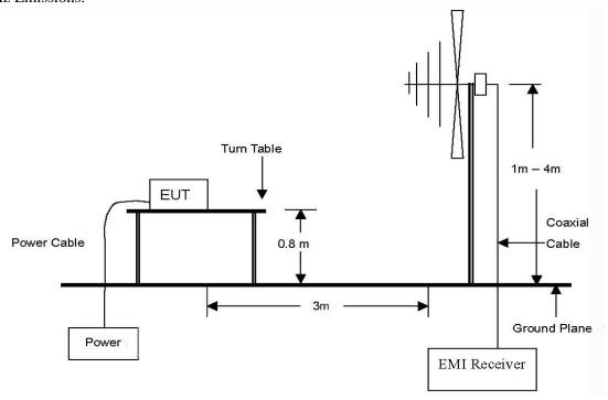
The diagram below shows the test setup that is utilized to make the measurements for emission from 1 GHz to 18 GHz Emissions.
