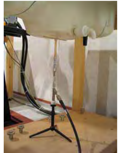
Photo of the dipole Antenna
