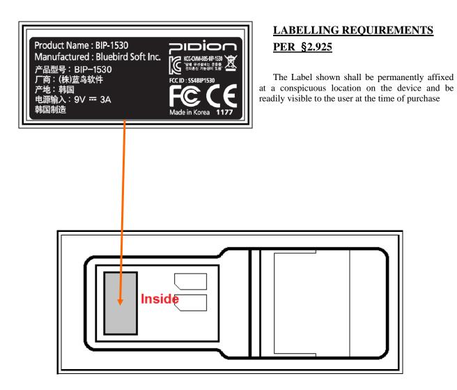
The label is attached to this device by an adhesive. The adhesive is permanent type with strong strength. Additionally, the label is readily to the purchaser at the time of purchase.
