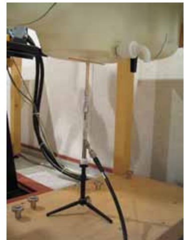
Photo of the dipole Antenna
