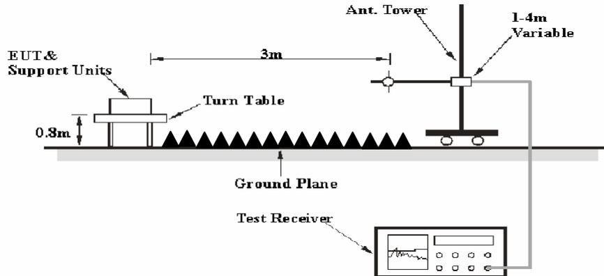
The radiated emission tests were performed in the 3 meters chamber test site, using the setup accordance with the ANSI C63.4-2003. The specification used was the FCC 15.209, and FCC 15.247 limits.
