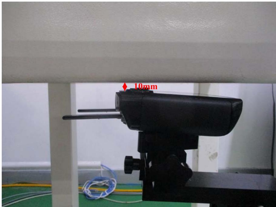
**Test Position\_Front Antenna Fold (10mm)**
