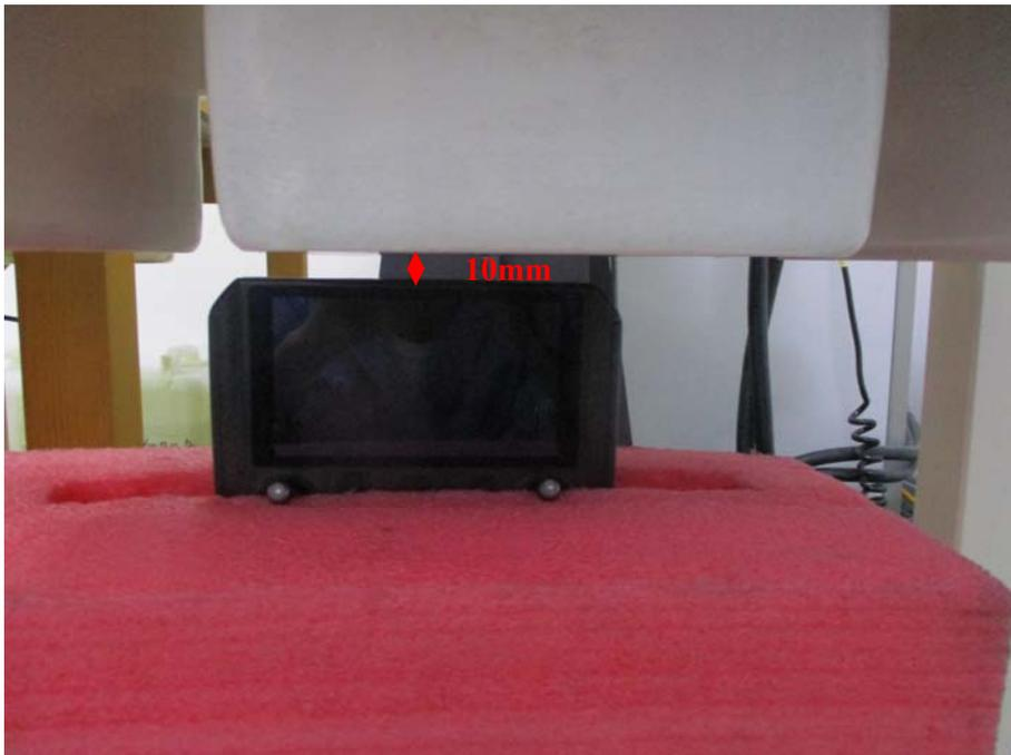
**Test Position\_Bottom(BT) (10mm)**
