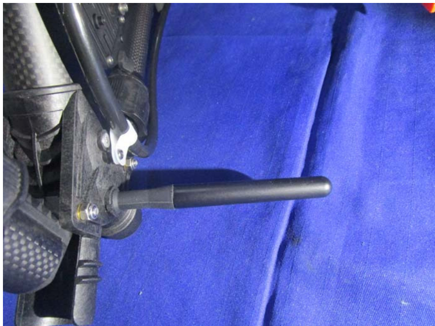
EUT – SDR Antenna View
