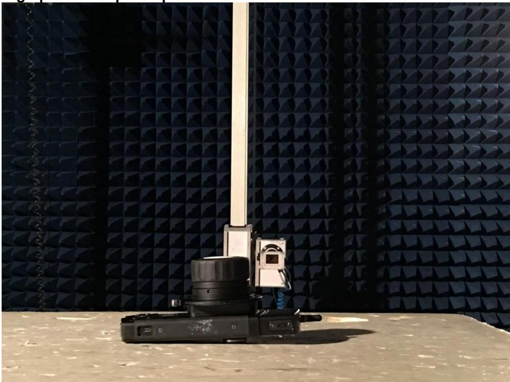
**Photograph 5: Set-up for Spurious Emissions of 26.5 – 40GHz**
