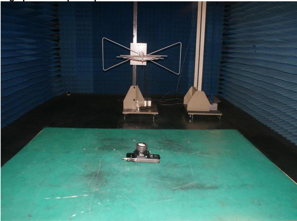
**Photograph 3: Set-up for Spurious Emissions of 1 – 18GHz**
