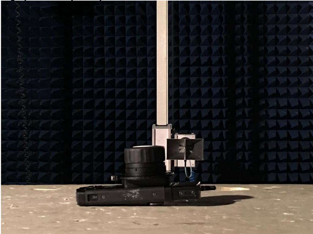
**Photograph 4: Set-up for Spurious Emissions of 18 – 26.5GHz**
