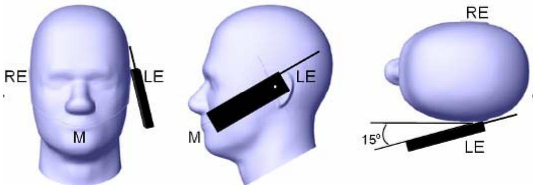
**Test positions for body-worn and other configurations**
