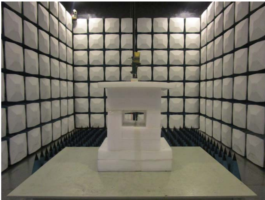
Radiated Emission Battery Mode View (Above 1GHz)
