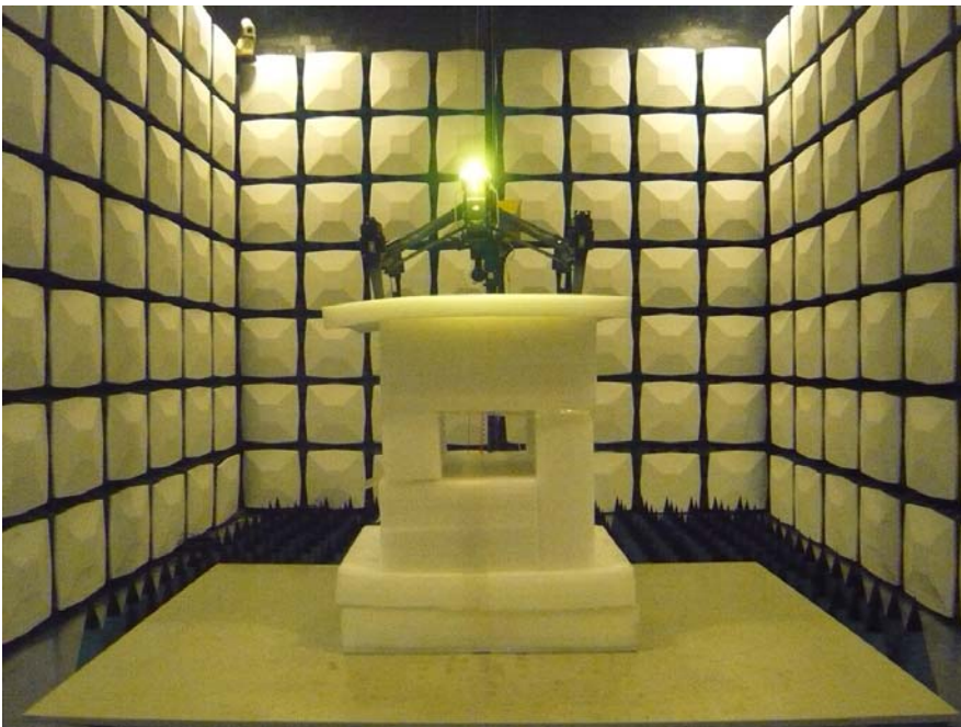
Radiated Emission Above 1GHz View
