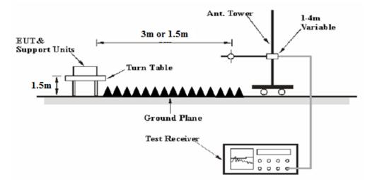
The radiated emission tests were performed in the 3 meters chamber, using the setup accordance with the ANSI C63.10-2013. The specification used was the FCC 15.209, and FCC 15.407 limits.
