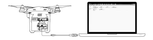
$\Lambda$  The aircraft must be turned on before attempting to access the files on the Micro-SD card.
