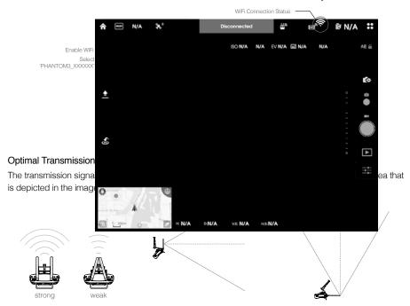
Ensure that the aircraft is flying within the optimal transmission zone. To achieve the best transmission performance, maintain the appropriate relationship between the operator and the aircraft.
