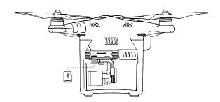
O Do not remove the Micro-SD card from the Phantom 3 4K when it is turned on.
