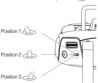
P-mode (Positioning): P-mode works best when the GPS signal is strong. There are three different versions of P-mode, which will be automatically selected by the Phantom 3 4K depending on GPS signal strength and the Vision Positioning sensors:
