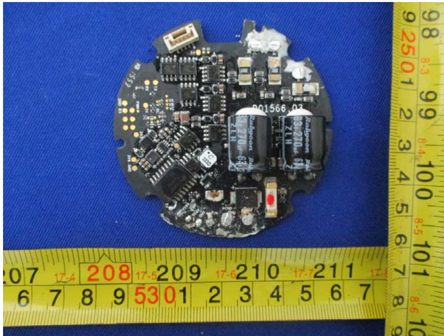
EUT – Motor Control Board Bottom View
