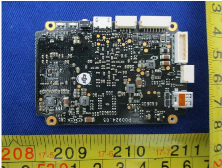
EUT – RF Module Driver Board Bottom View
