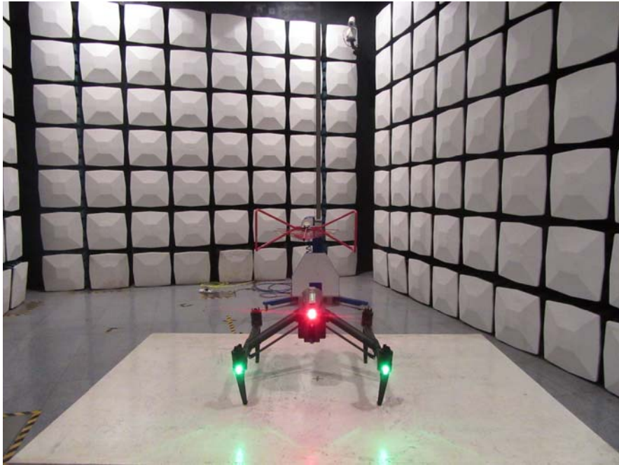
Radiated Emission View (Below 1GHz)
