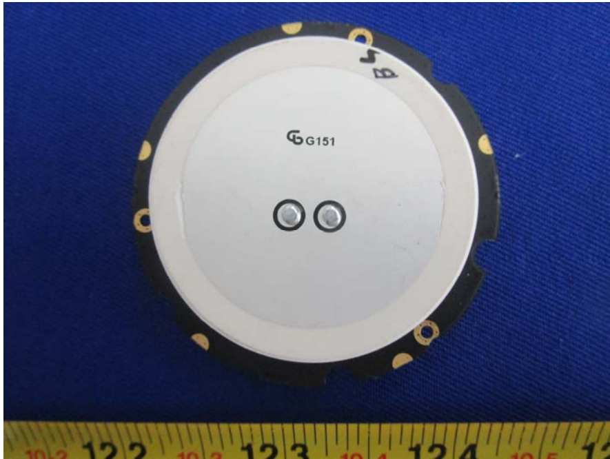
EUT – GPS Module Top & Antenna View
