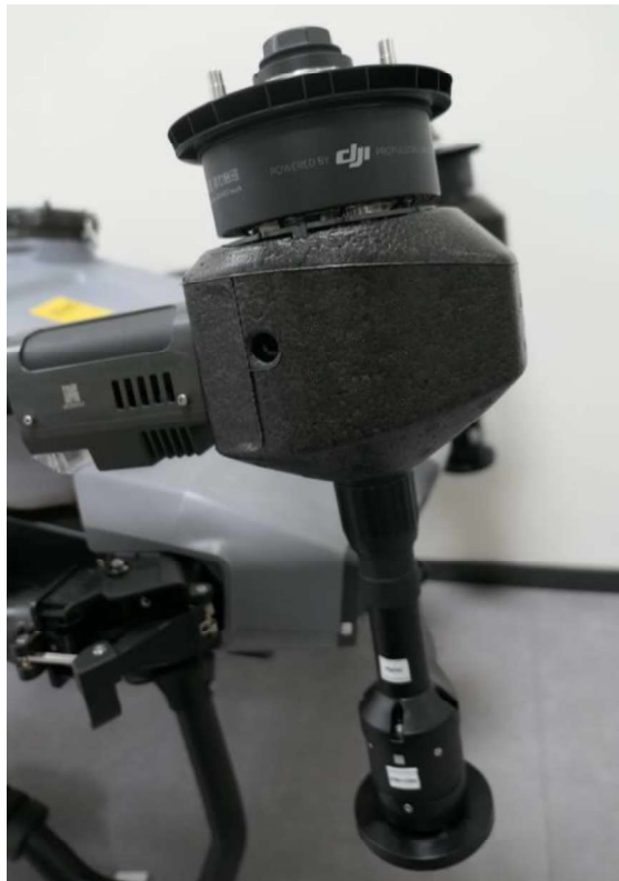
Fig. 46: Rear propeller mechanism and spray mechanism view -1 (for model 3WWDZ-20A)
