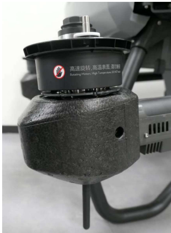
Fig. 44: Front propeller mechanism view -1 (for model 3WWDZ-20A)
