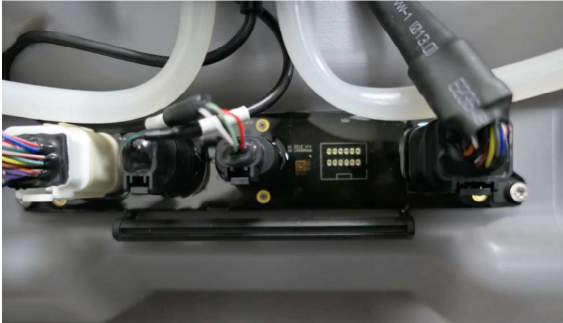
Fig. 43: Terminal board for spray module (for both models)
