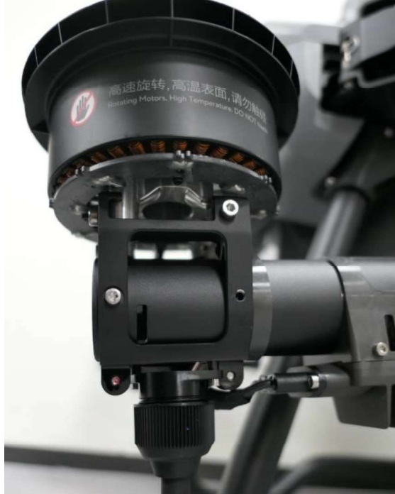
Fig. 45: Front propeller mechanism view -2 (after foam removed, for model 3WWDZ-20A)
