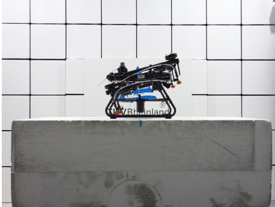
Photograph 1: Test Setup for Spurious Emissions (Front View 1)
