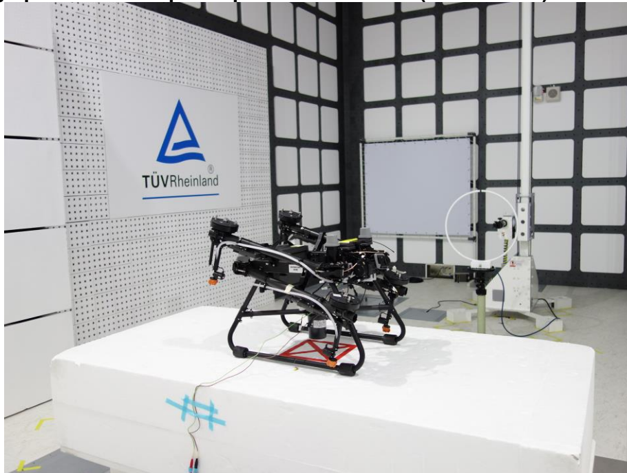
Photograph 6: Test Setup for Spurious Emissions (Back View 4)
