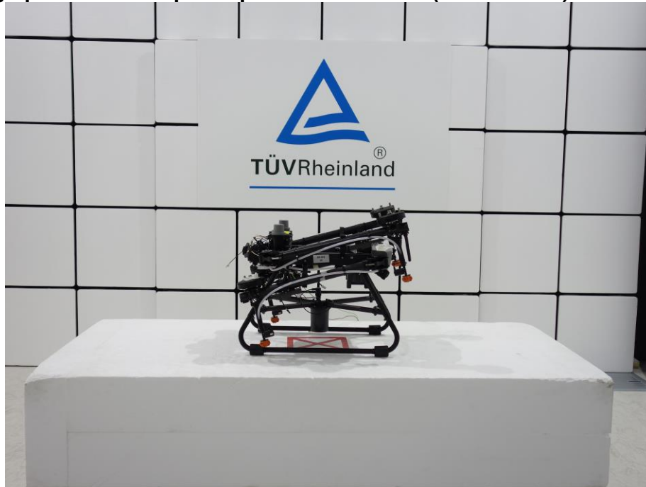
Photograph 2: Test Setup for Spurious Emissions (Front View 2)
