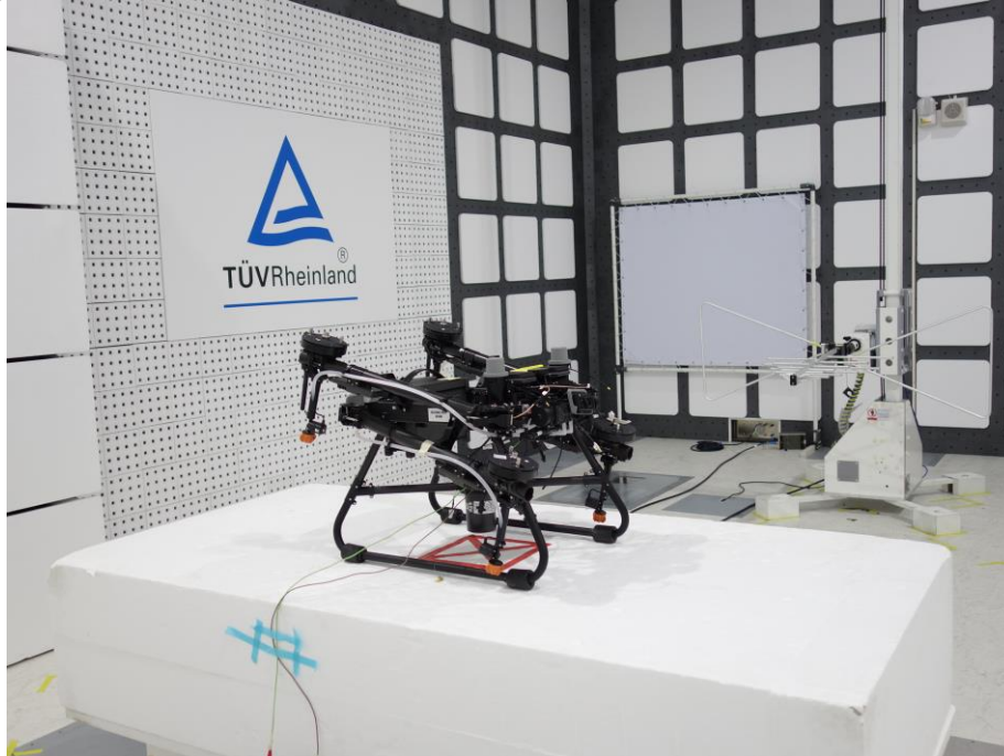
Photograph 5: Test Setup for Spurious Emissions (Back View 3)
