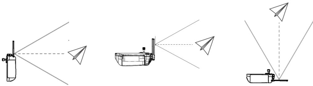
The optimal transmission range is where the antennas are facing toward the aircraft and the angle between the antennas and the back of the remote controller is 180° or 270°.
