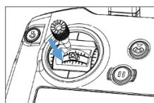
Attach the control sticks and twist to secure
