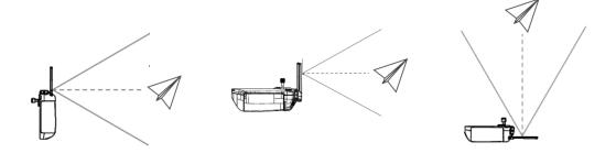
The optimal transmission range is where the antennas are facing toward the aircraft and the angle between the antennas and the back of the remote controller is  $180^{\circ}$  or  $270^{\circ}$ .
