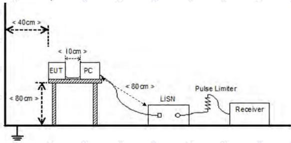
The EUT is placed on a 0.8m high insulating table, which stands on the grounded conducting floor, and keeps 0.4m away from the grounded conducting wall. The EUT is connected to the power mains through a LISN which provides  $50\Omega/50\mu H$  of coupling impedance for the measuring instrument. A Pulse Limiter is used to protect the measuring instrument. The factors of the whole test system are calibrated to correct the reading.
