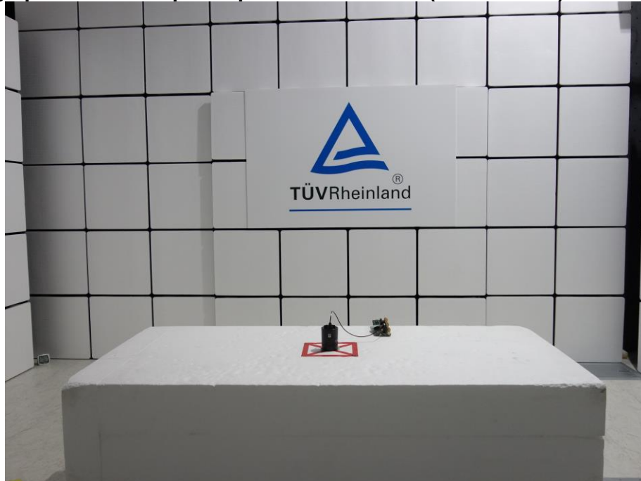
Photograph 2: Test Setup for Spurious Emissions (Front View 2)
