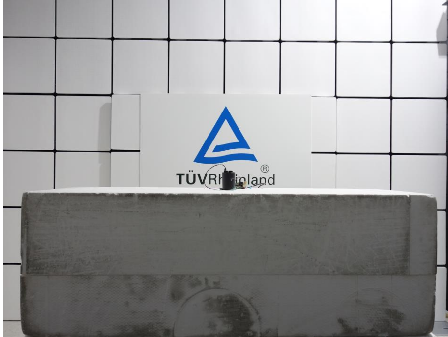
Photograph 1: Test Setup for Spurious Emissions (Front View 1)
