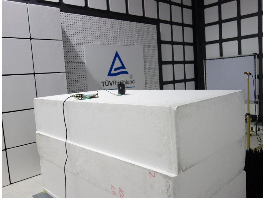
Photograph 5: Test Setup for Spurious Emissions (Back View 3)
