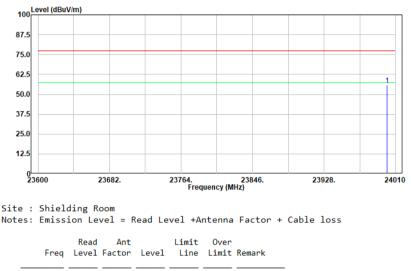
MHz dBuV dB/m dBuV/m dBuV/m dB 1 24000.000 31.11 39.23 55.69 77.48 -21.79 Peak
